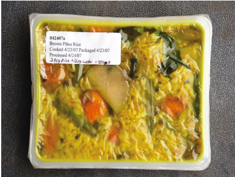
Fig. 11.10 Prototype of shelf-stable prepared meal ready-to-eat in retortable microwavable semi-rigid tray with transparent lid stock (Reproduced from Rich 2007 with permission)
