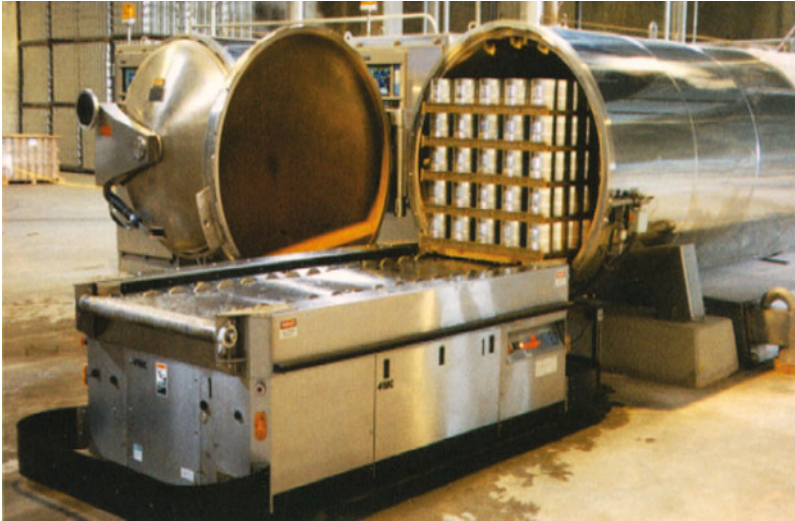
Fig. 11.5 Automated Guided Vehicle in process of retort loading/unloading (Photo courtesy of JBT FoodTech, formerly FMC FoodTech, Madera, CA)
