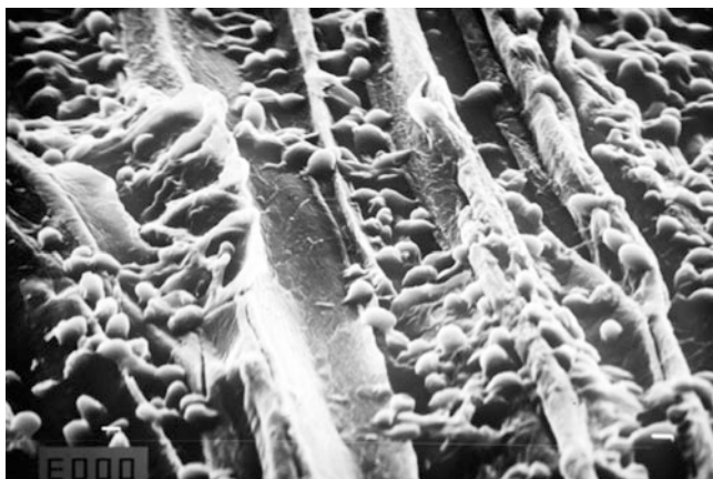
Fig. 6.1 Scanning electron microscope (SEM) photo of yeast cells immobilized on wood chips
