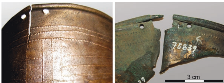
Fig. 9.11 Wear marks on greaves. Left : Lengyeltóti, Hungary; crack with two rivet holes punched from the inside. Right : Stetten/Teiritzberg, Austria (Prähistorische Abteilung NHM Wien). In this greave, too, the holes were punched from the inside to host a wire holding the two sides of the crack together. (Photographs: M. Mödlinger)
