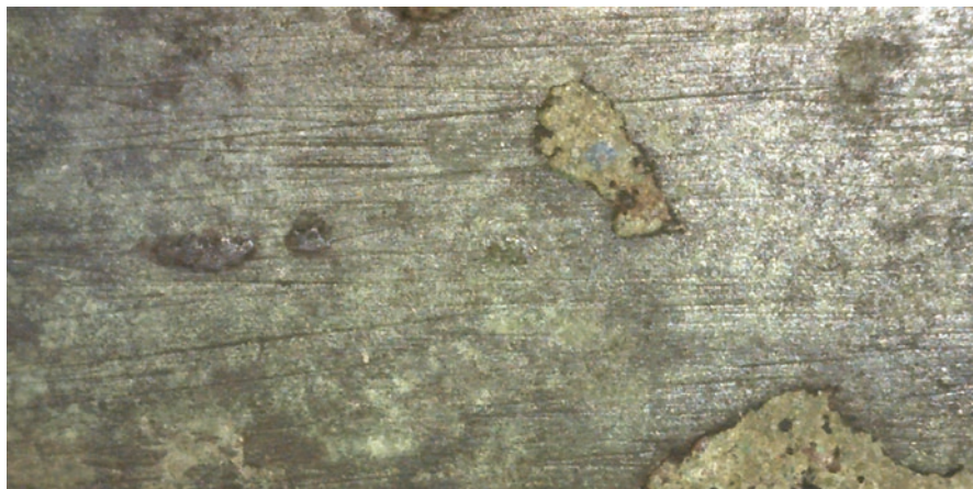
Fig. 11.6 Striations partially covered by corrosion products (ID 7)
