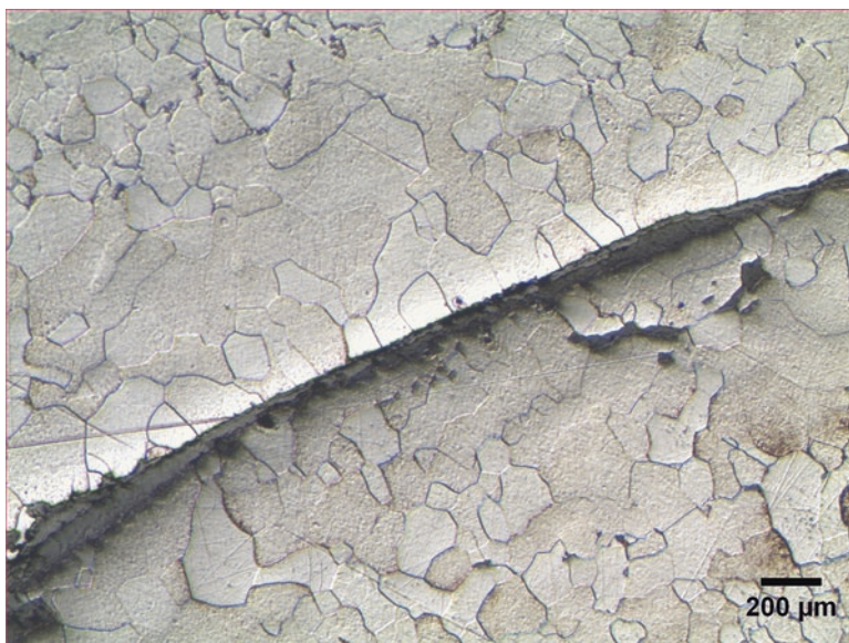
Fig. 12.6 Photo micrograph of a weld line in lance E2295, showing mostly recrystallised ferrite and some agglomerate grains along the seam (CLR 50×)
