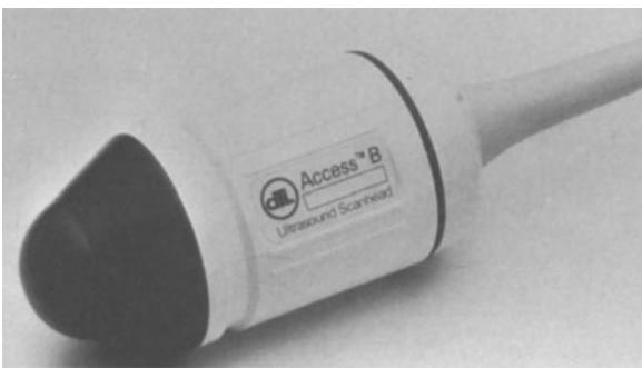
Rotating probe Annular array 3 cm Ø 3–10 MHz (ATL)
