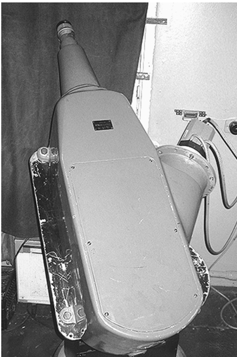
Fig. 3.5 The SP-50 spectrograph with the FPZS INSTASPEC IV unit
