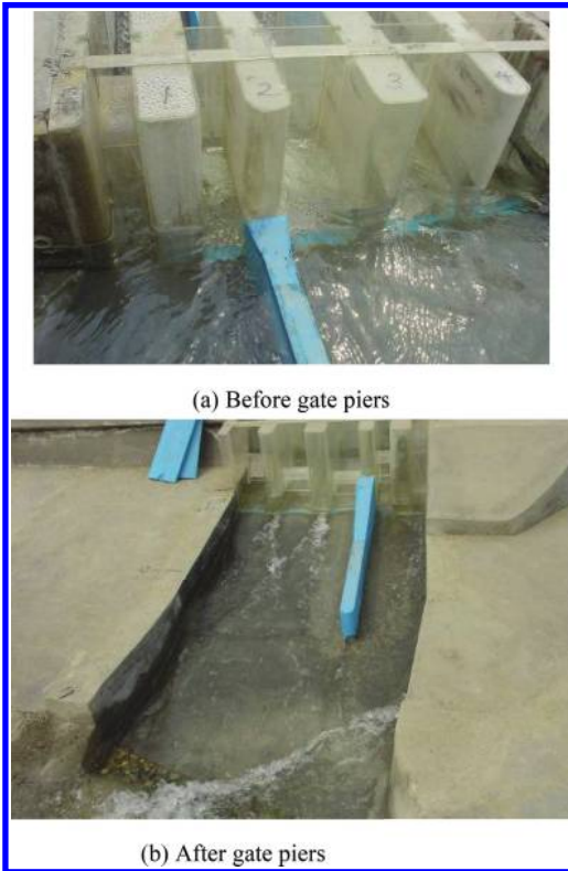
Figure 3. Flow pattern at the check discharge.
