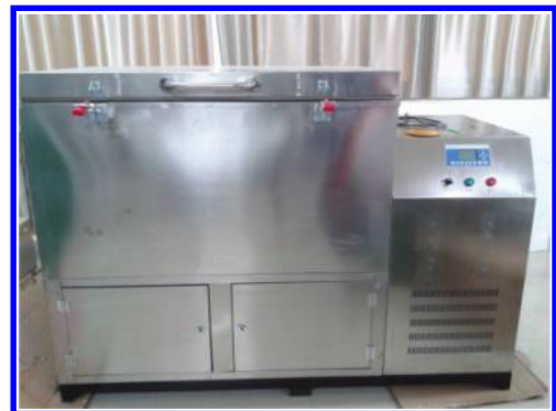
Figure 3. Freeze-thaw test machine.
