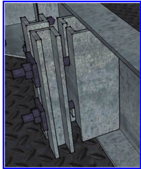
Figure 9. Conjunction node three-dimension of the window mold.
