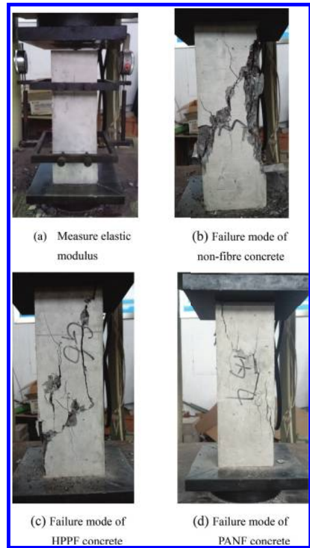
Figure 3. Elastic modulus measurement and failure mode of three kinds of concrete.
