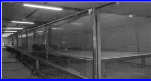
Figure 1. Reduced-scale model tunnel.
