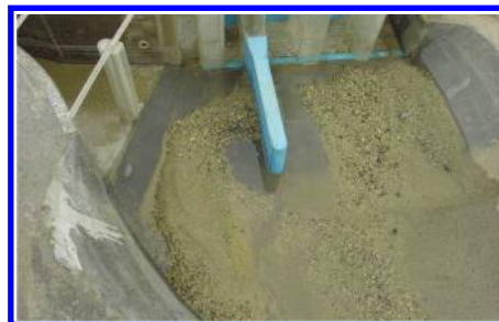
Figure 2. Deposit of the sediment after 12-hour scours at the check discharge.
