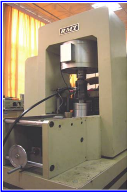
Figure 1. Testing machine of RMT-201.
