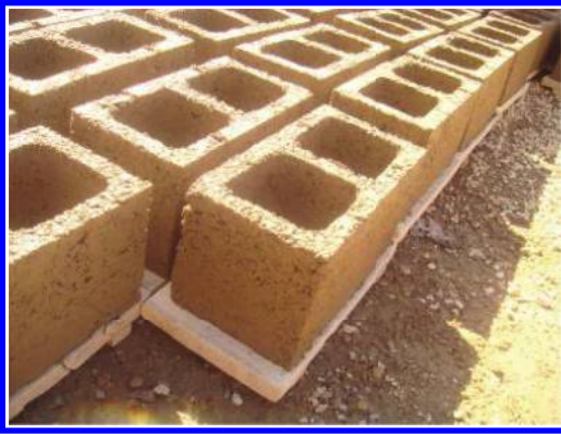
Figure 5. Slag hollow bricks made in Nu-River basin.
