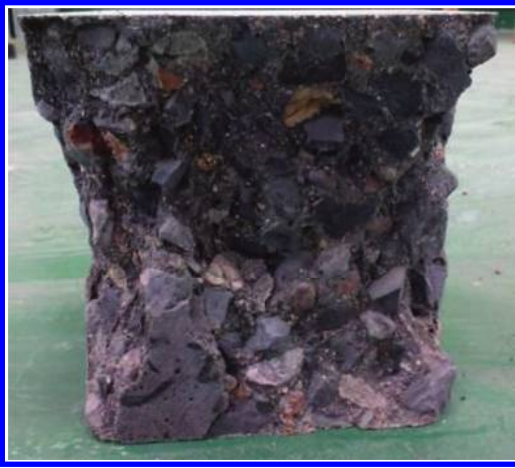
Figure 6. Failure mode of cubic specimen.
