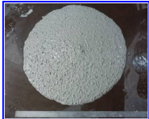
Figure 4. Slump flow of PSC-SCC.
