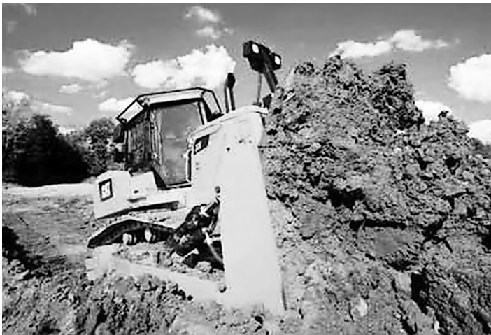
Figure 10-18. Caterpillar D7E Electric Dozer
