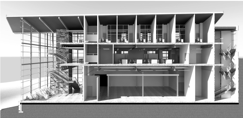
Figure 9-6. BIM Rendering of Section of Office Building
