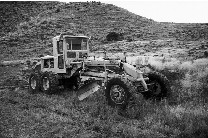
Figure 4-9. Old Heavy Construction Equipment Motor Grader
