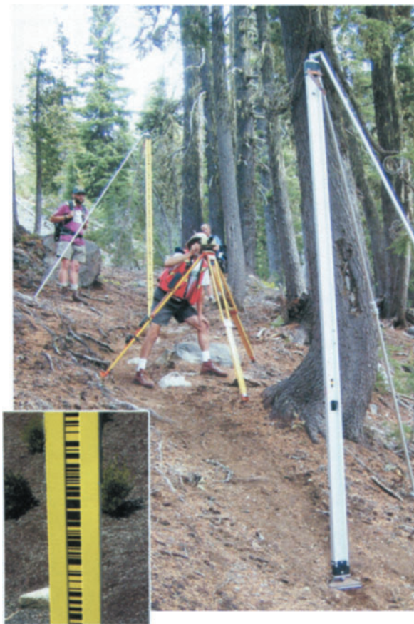
Figure 2.25. Leveling in backcountry terrain can be physically challenging but nonetheless rewarding for a hardy crew. Here, a Leica NA 3003 digital level and barcode rods ( inset ) are used to level along a trail in the Three Sisters Wilderness, Oregon. USGS photograph by Michael P. Poland.
