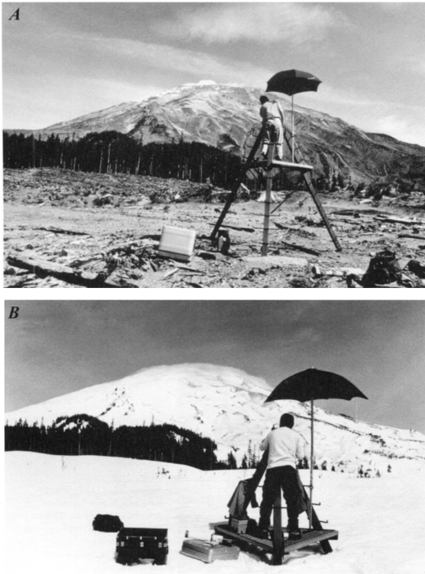
Figure 2.10. (A) EDM station Clearcut at Mount St. Helens in summer. (B) Same station in winter with \sim 2 m snowpack. USGS photographs by Lyn Topinka, reprinted from Iwatsubo et al. (1992a).
