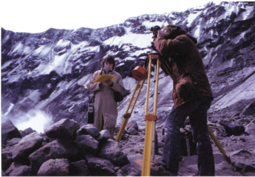
Figure 2.21. Using a theodolite to measure horizontal and vertical angles in the 1980 crater at Mount St. Helens. Under ideal conditions, the precision of such measurements is \pm 1 arc second, which corresponds to a displacement of \pm 5 mm at a distance of 1 km. Displacement vectors for a set of targets can be derived from repeated measurements from two or more theodolite stations by assuming that the theodolite stations did not move. USGS photo by Daniel Dzurisin, 20 May 1982.
