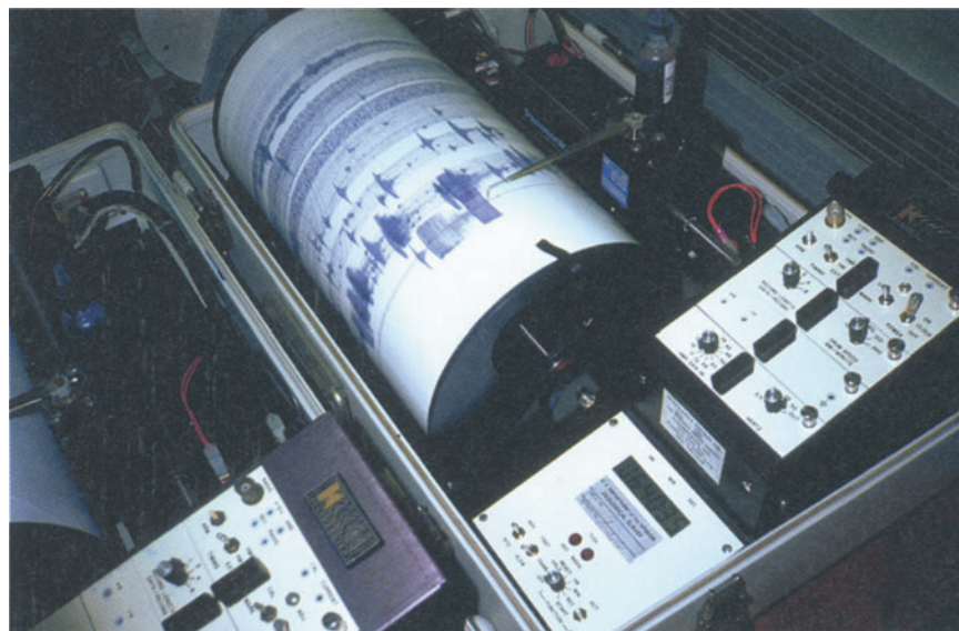
Figure 1.10. Kinemetrics Inc. PS-2 portable drum recorder showing the onset of a swarm of earthquakes at Soufriere Hills Volcano, Montserrat, West Indies. A small network of seismographs, telemetry links, recorders, and an automated data-analysis system can be installed quickly during a volcano crisis to provide essential seismic information in real time. USGS photograph by C. Daniel Miller, August 1995.
