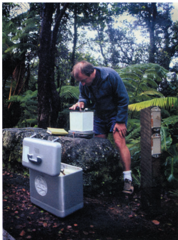
Figure 1.17. Geophysicist Daniel J. Johnson makes a precise gravity reading with a LaCoste & Romberg portable gravimeter at a station near Thurston Lava Tube, Kīlauea Volcano, Hawai'i. Photograph by Eileen Llona.
