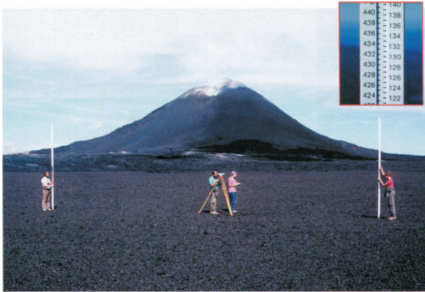
Figure 2.24. Leveling near the Pu'u 'Ō'ō vent along the East Rift Zone of Kīlauea Volcano, Hawai'i, using an optical level and dual-scale Invar rods ( inset ). Modern levels are capable of measuring the height difference between graduated rods in a single set-up to a precision of 0.1 mm or better. Using such an instrument, an experienced crew can cover 3–5 km day -1 in relatively flat terrain, or 1–3 km day -1 in steeper terrain. USGS photograph by James D. Griggs, 12 January 1985.
