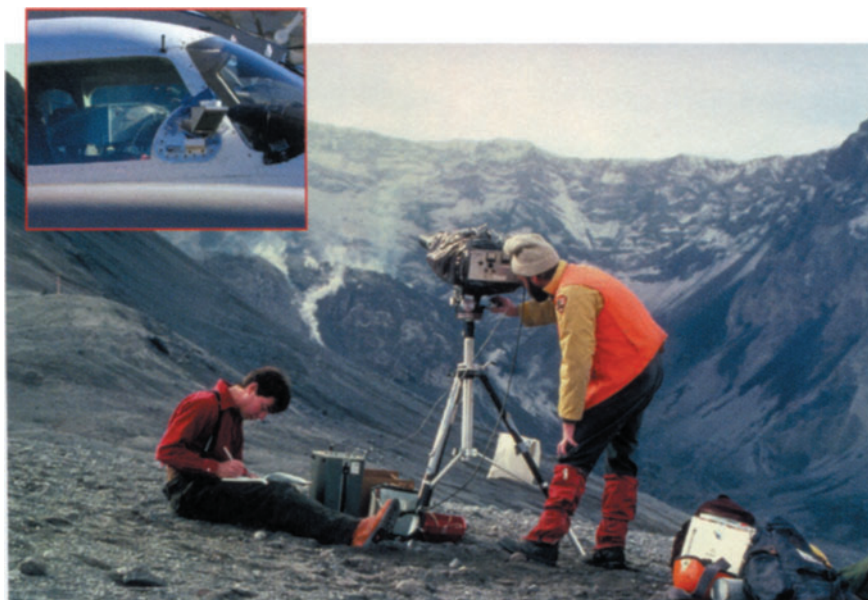
Figure 1.12. A COSPEC can be used to measure the concentration of sulfur dioxide ( \text{SO}_2 ) gas in a volcanic plume. The instrument can be mounted on a tripod, on a wheeled vehicle, or on an aircraft ( inset ). COSPEC measurements can be combined with wind-speed data to calculate the emission rate of \text{SO}_2 , which sometimes is a good indicator of shallow magma intrusion. USGS photographs by Lyn Topinka and Kenneth A. McGee ( inset ).
