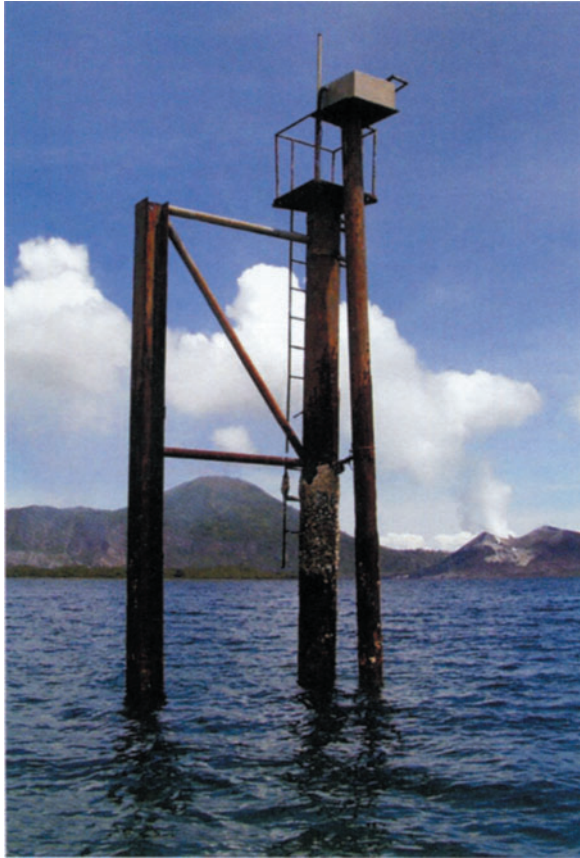
Figure I.4. Tide gauge on the eastern side of Vulcan, a vent located along the western ring fracture of Rabaul Caldera, Papua New Guinea. The gauge was lifted nearly out of the water during the night preceding the start of simultaneous eruptions at Vulcan and Tavurvur, which can be seen venting in the background. Before the 1994 eruptions, mean sea level was approximately at the third step of the ladder, as marked by the top of the light-colored accumulation of mussel shells. USGS photograph by Elliot T. Endo, November 1999.
