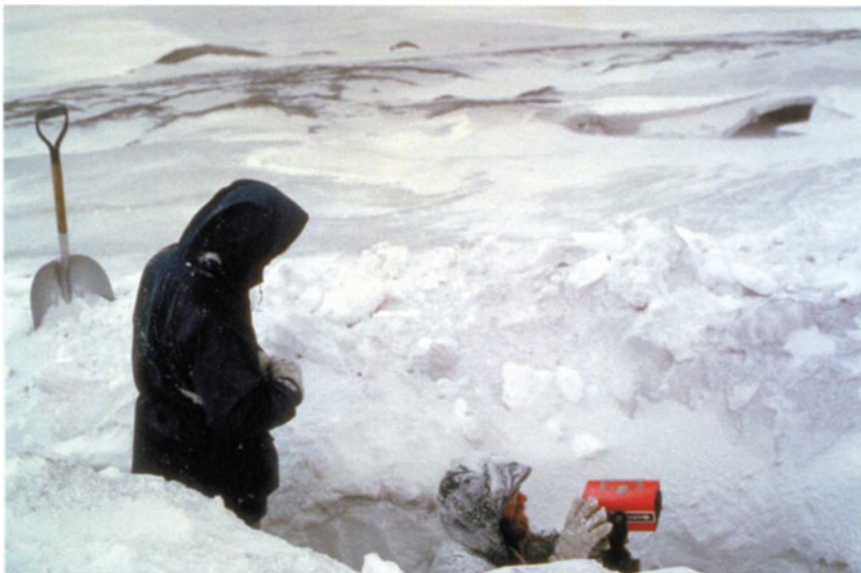
Figure 2.8. Wintertime EDM survey at station Sauna in the crater at Mount St. Helens. USGS photograph by Lyn Topinka, 22 March 1983.
