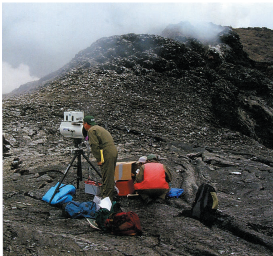
Figure 1.14. Scientists use an open-path FTIR spectrometer to measure the concentrations of volcanic gases from vents along the East Rift Zone of Kīlauea Volcano, Hawaii. This instrument can determine the concentrations of many common magmatic gases, including \text{SO}_2 , \text{CO}_2 , \text{CO} , \text{COS} , \text{HCl} , and \text{HF} . USGS photograph by Michael P. Doukas.
