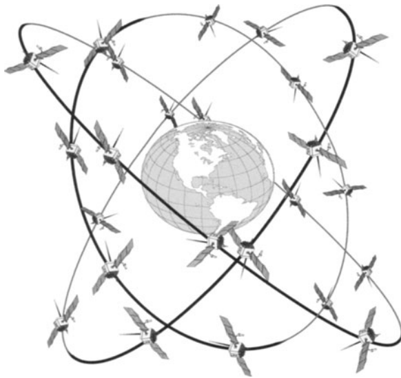
Figure 4.2. The Russian GLONASS satellite constellation, which when fully deployed includes 24 satellites in 3 orbit planes. FOC was achieved in January 1996, but the number of operating satellites has since declined. See Table 4.1 for additional details.
