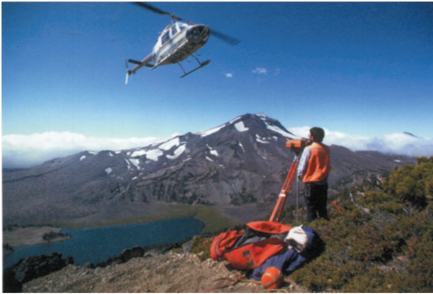
Figure 2.5. EDM survey at South Sister Volcano in the Three Sisters region, central Oregon. A Hewlett-Packard 3808A infrared EDM is used to measure line length while a helicopter flies along the line-of-sight making refractivity measurements. A fixed-wing aircraft can also be used for this purpose. USGS photograph by Lyn Topinka, 1985.
