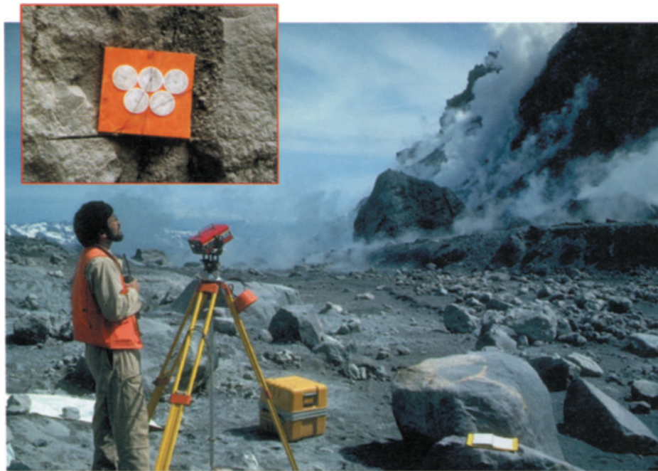
Figure 2.4. Line-length monitoring in the 1980 crater at Mount St. Helens. A Lietz Red IA EDM is set up over a survey point on the crater floor to measure distances to fixed reflectors on the lava dome (steaming, upper right). During the period of dome growth from 1980 to 1986, inexpensive highway reflectors (inset) or single corner cube reflectors were used for this purpose; repeated measurements could be made without visiting the reflectors each time. The practice was also a money saver, because reflectors were destroyed frequently by rock-falls or eruptive activity and had to be replaced (Iwatsubo and Swanson, 1992). EDMs like this one can measure line lengths up to several kilometers with an accuracy of the order of [(5 \text{ mm})^2 + (1 \text{ mm/km} \times L(\text{km}))^2]^{1/2} (i.e., \pm 11 \text{ mm} for a 10 km line). USGS photograph by Steven R. Brantley, 9 June 1982.
