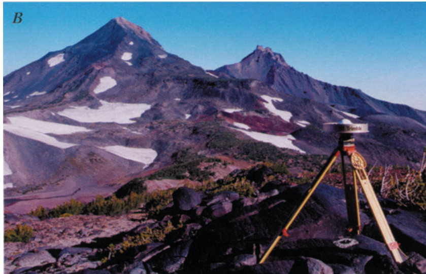
Figure 4.3. (A) Trimble model 4000 SSE GPS receiver and antenna set up at bench mark HVO88-14 on Poli'ahu Cone near the summit of Mauna Kea Volcano, Hawai'i. Hualalai Volcano is visible in the distance. (B) Trimble choke-ring antenna set up at bench mark CVO 85-308 on the north flank of South Sister Volcano, Oregon. A Trimble model 4000 SSI GPS receiver, which is connected to the antenna by a cable on the right, is not visible in the photograph. Middle Sister (left) and North Sister (right) can be seen in the distance. (A) USGS photograph by Maurice K. Sako. (B) USGS photograph by David E. Wieprecht, 19 October 2001.
