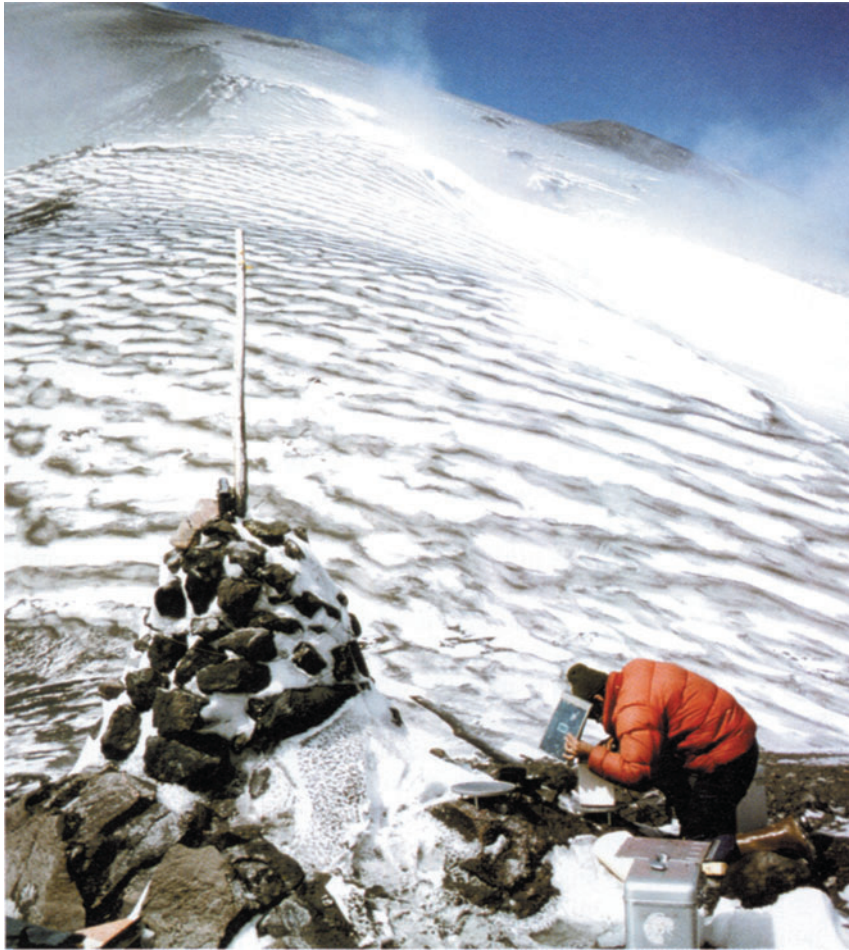
Figure 2.38. The author using a gravity meter at East Dome on the east flank of Mount St. Helens during a small phreatic eruption in April 1980. Ash covering snow is from a series of such eruptions that preceded the large debris avalanche and magmatic eruption on 18 May 1980. At each gravity station, measurements were made at two sites separated by no more than a few meters with each of two LaCoste & Romberg gravimeters. This redundancy made it easier to identify measurement errors or instrument tares (Jachens et al. , 1981). USGS photograph by Carter W. Roberts.
