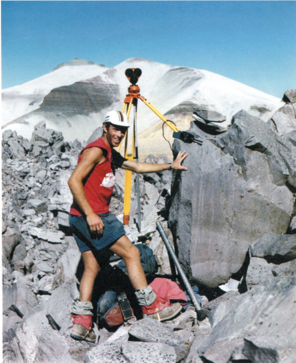
USGS scientist Jack Kleinman, typically attired in shorts and a smile, sets up EDM reflectors on Novarupta lava dome in the Valley of Ten Thousand Smokes, Alaska, with Baked Mountain in the distance. The rhyolite dome was emplaced during the waning phase of the largest volcanic eruption of the 20th century, which produced about 20 \text{ km}^3 of air-fall tephra and 11\text{--}15 \text{ km}^3 of ash-flow tuff within about 60 hours in June 1912. Jack helped to establish a geodetic network near Novarupta in 1989 and served as crew chief for follow-up surveys in 1990 and 1993. His energy and zest for life inspired all those who knew him. Jack died in a kayaking accident on the White Salmon River, Washington, in 1994. Photograph by John Eichelberger, University of Alaska Fairbanks.
