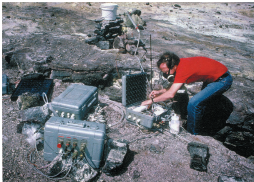
Figure 1.15. Gas and temperature monitoring station in the summit area of Kīlauea Volcano, Hawai‘i. Commercially available chemical sensors have been modified to operate in harsh volcanic conditions, thus providing a continuous record of the concentrations of several fumarolic gases. USGS photograph by James D. Griggs.
