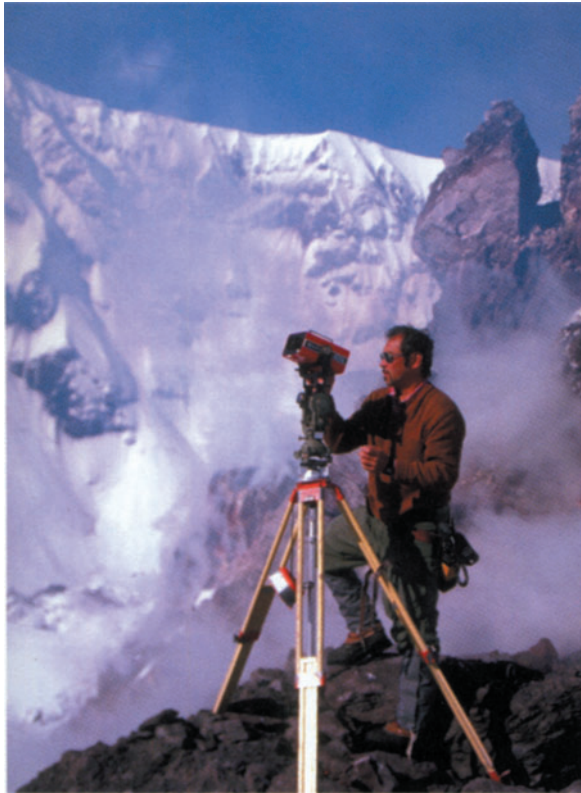
Figure 2.23. Line-length and angular measurements can be made in tandem by mounting an EDM and conventional (i.e., non-electronic) theodolite together on a tripod. Here, such a set-up is being used on the lava dome at Mount St. Helens, with the snow covered wall of the 1980 crater in the distance. USGS photograph by Steven R. Brantley, March 1986.
