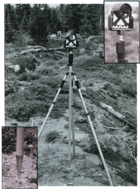
Figure 2.31. Reflector target for single-setup trigonometric leveling set up over an expansion bolt ( lower inset ) in a lava flow (Ewert, 1992). The target-cross and prism are set apart vertically ( upper inset ) the same distance as the theodolite telescope and EDM (Figure 2.30).
