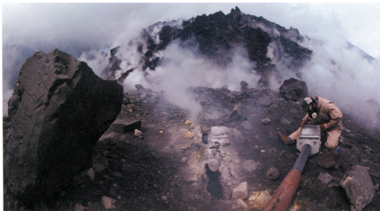
Figure 1.22. The author inspects a crack meter on the crater floor at Mount St. Helens. A wire is stretched across the crack inside a pipe and attached to anchor points on either side. Changes in the length of wire played out between the anchor points are sensed by a linear displacement transducer and converted to a digital signal inside the box. A radiotelemetry system (not shown) transmits the signal to the USGS David A. Johnston Cascades Volcano Observatory in Vancouver, Washington. A dacite lava dome that grew in the crater from 1980 to 1986 steams in the background. Photograph reprinted with permission from photographer Steve Raymer and the National Geographic Society.
