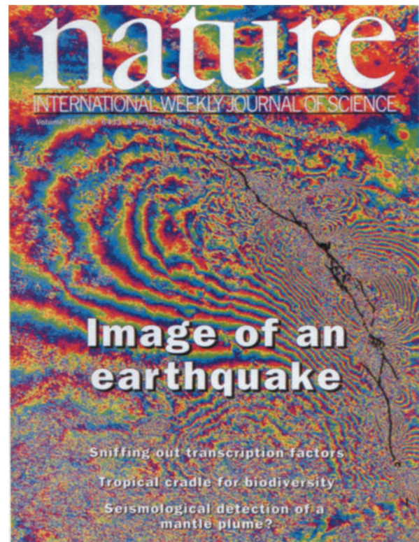
Figure 5.2. This historic satellite radar interferogram, which appeared on the cover of the 8 July 1993 issue of Nature , depicts in remarkable detail surface displacements caused by the M 7.3 Landers, California, earthquake on 28 June 1992 (Massonnet et al. , 1993). Each color cycle from violet to red represents 2.8 cm of slant-range change. Black lines indicate the fault geometry as mapped in the field. Reprinted by permission from Nature , volume 364, no. 6433, 8 July 1993, copyright 1993 Macmillan Publishers Ltd.
