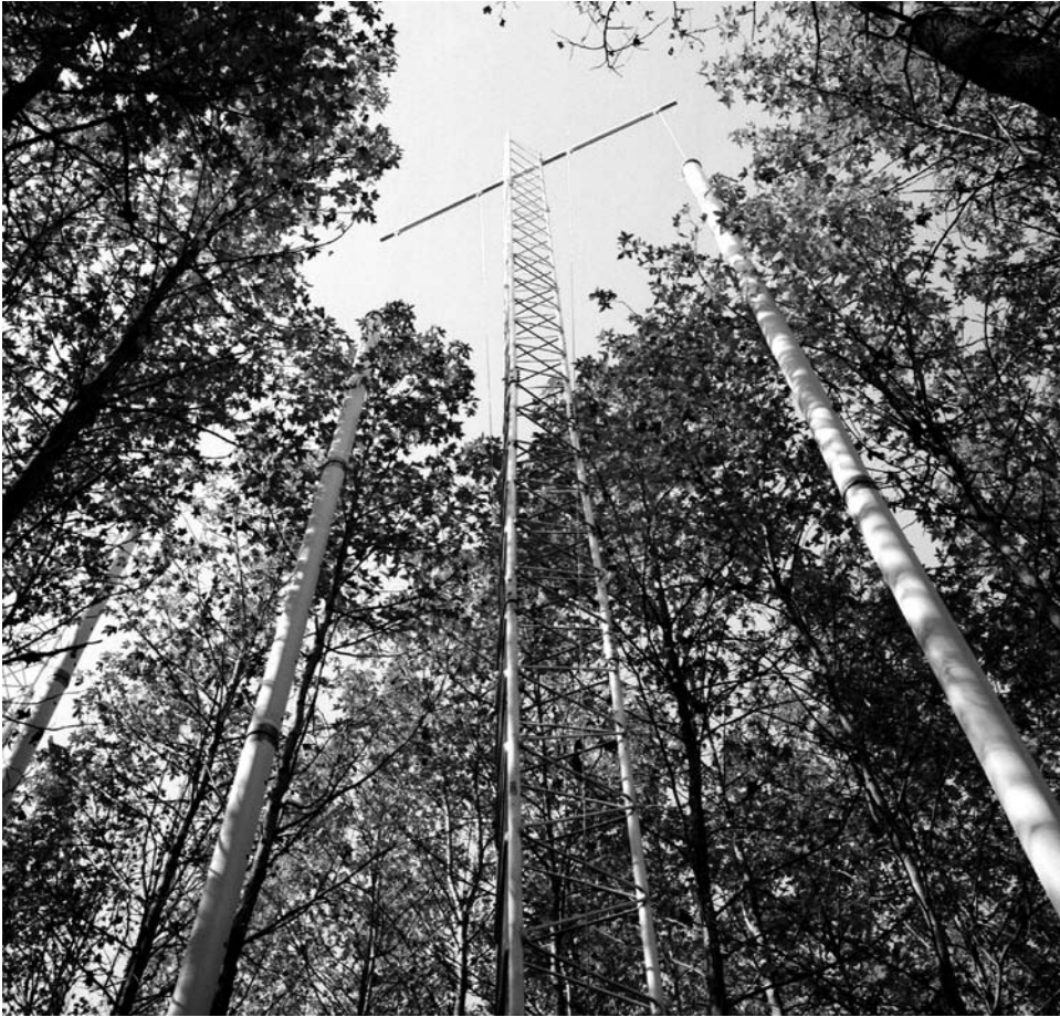
Figure 8.3. The Tennessee FACE site showing the towers used to release CO 2 into the forest. Source: Rich Norby/ORNL FACE.
