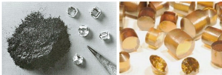
Fig. 11.1 Graphite and diamond (from D. a. Mcqurie and P. A. Rock, “Descriptive Chemistry” W.H. Freeman and Co., 1985), and an artificially synthesized diamond (called “HIME-diamond” http://www.47news.jp/CN/201012/CN2010121801000015.html )
