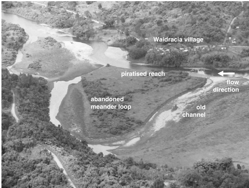
FIG. 10.4. Low-level aerial view in July 2001 of the Wainimala River adjacent to Waidracia village, in the Rewa basin, Fiji. Prior to early 2000, the river occupied the big meander loop in the centre of the photograph. A minor tributary channel originally flowed from right to left in front of the village, joining the main river farther downstream. Down-valley migration of the meander bend occurred during a high flow caused by rainfall associated with Tropical Cyclone Neil in mid-April 2000. This led to piracy of the tributary channel and abandonment of the old meander in preference for the present straight course. The area of floodplain farmland enclosed by the cut-off loop is now effectively 'lost' from Waidracia village ownership. Photo by Ray Kostaschuk.
