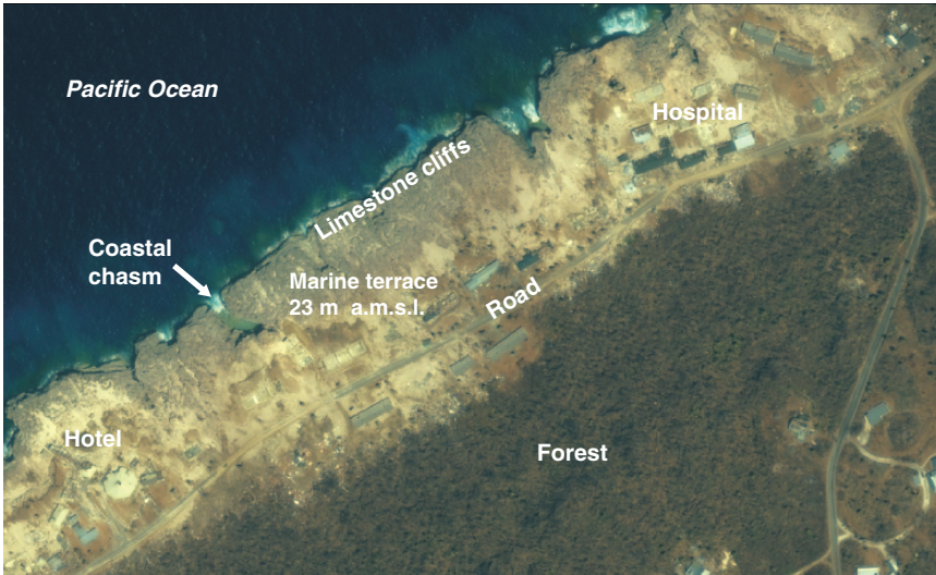
FIG. 7.12. Satellite image of the Niue coastline at the capital Alofi on the west coast. Immense waves generated by Tropical Cyclone Heta on 6 January 2004 overtopped the coastal cliffs, and scoured a zone to a distance of up to 200 m inland on the 23 m elevation marine terrace, flattening trees and buildings, including the hospital complex and the Niue Hotel. Base image courtesy of NOAA.
