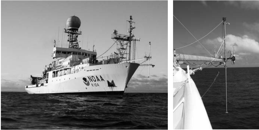
Figure 19.1. The boom system on the bow of the Ronald H. Brown research vessel (left) during the GasEx-2001 open ocean CO 2 exchange experiment in the equatorial Pacific (3°S 125°W). The boom was extended 10 m from the side of the vessel. Direct covariance and gradient CO 2 flux micrometeorological methods were performed when the bow was manoeuvred into the predominant wind direction. Vertical profiles of atmospheric CO 2 near the ocean surface were measured from the mast located at the end of the boom (right).
