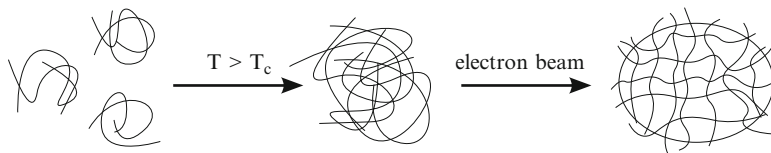
Fig. 5 Synthesis of PVME particles by irradiation of phase-separated solutions. Above the phase transition temperature T_c , the polymer chains collapse to globular aggregates. The collapsed structures are fixed by electron beam irradiation to yield temperature-sensitive microgel particles
