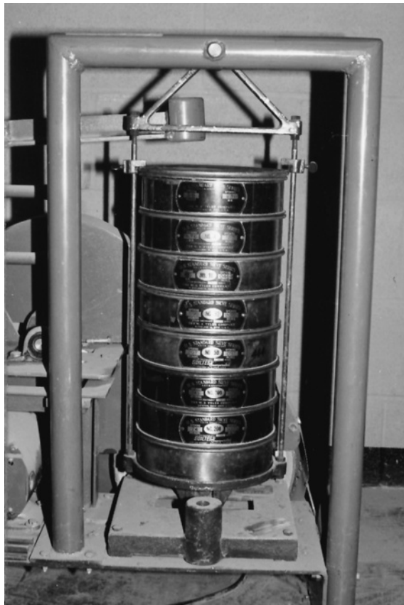
Figure 2.26 A set of sieves for a test in the laboratory (Courtesy of Braja M. Das, Henderson, Nevada)
