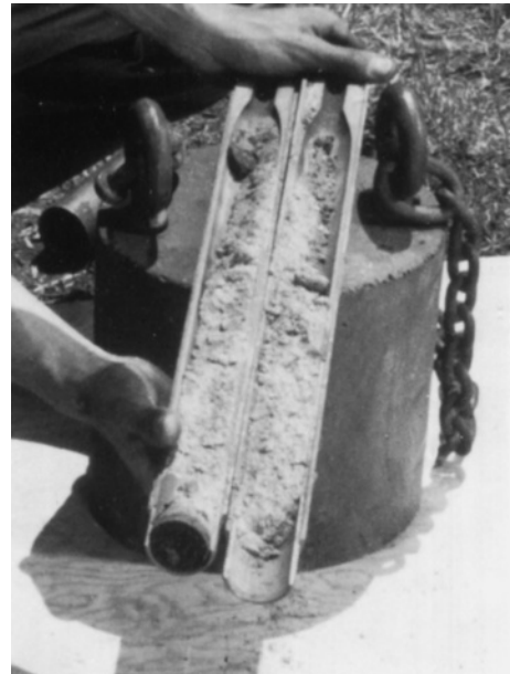
Figure 17.6 Split-spoon sampler, unassembled (Courtesy of ELE International)
