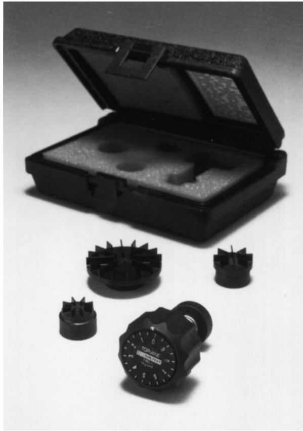
Figure 12.49 Torvane (Courtesy of ELE International)
