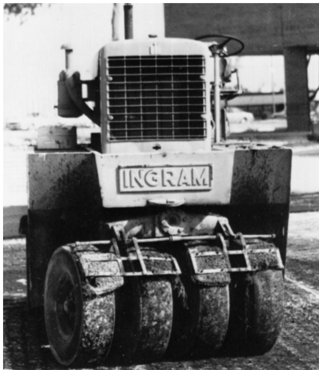
Figure 6.16 Pneumatic rubber-tired roller ( Ingram Compaction LLC )
