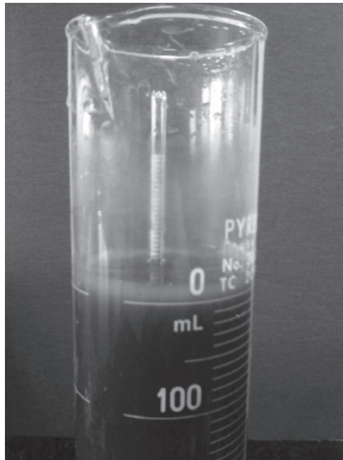
Figure 2.29 ASTM 152H type of hydrometer placed inside the sedimentation cylinder (Courtesy of Khaled Sobhan, Florida Atlantic University, Boca Raton, Florida)
