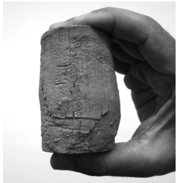
Figure 12.38 Failure by bulging of an unconfined compression test specimen (Courtesy of Braja M. Das, Henderson, Nevada)
