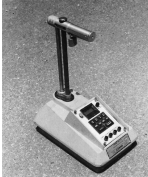
Figure 6.26 Nuclear density meter (Courtesy of Braja M. Das, Henderson, Nevada)
