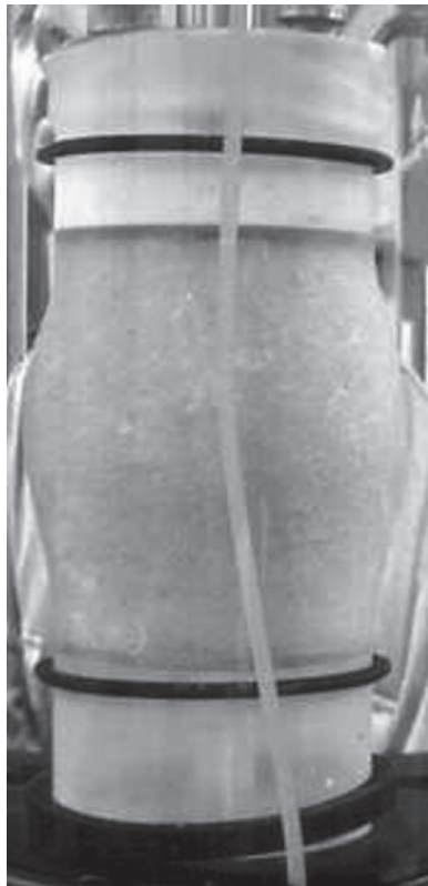
Figure 12.29 Triaxial soil specimen at failure during a consolidated-undrained test (Courtesy of S. Varapalli, University of Ottawa, Canada)
