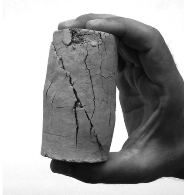
Figure 12.37 Failure by shear of an unconfined compression test specimen (Courtesy of Braja M. Das, Henderson, Nevada)
