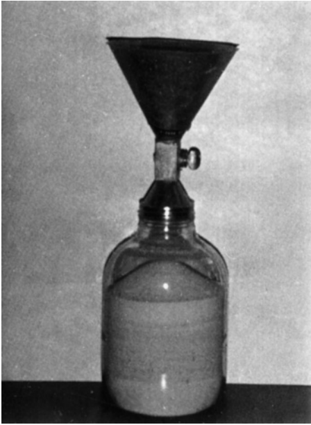
Figure 6.23 Glass jar filled with Ottawa sand with sand cone attached (Courtesy of Braja M. Das, Henderson, Nevada)
