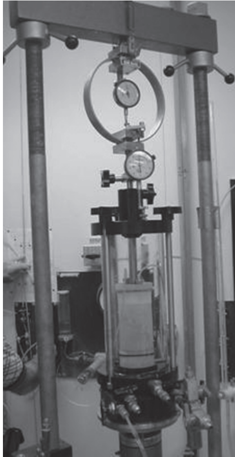
Figure 12.21 A triaxial test in progress in the laboratory (Courtesy of S. Vanapalli, University of Ottawa, Canada)
