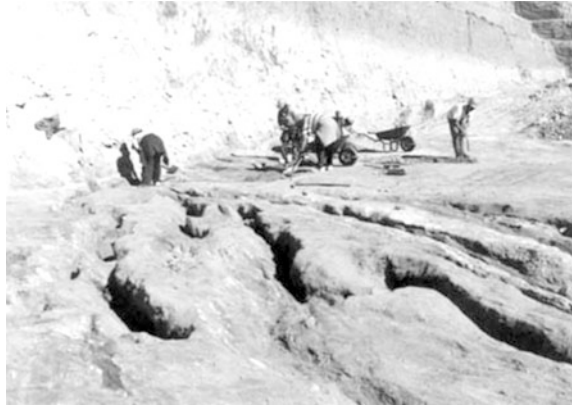
Fig. 7.4 An alluvial diamond mine on an old beach terrace. The diamonds are trapped in grooves in the bedrock. Image courtesy of Diamond Fields International ( http://www.diamondfields.com/s/Namibia.asp?reportID=88890 , [accessed on 5 April 2016])
