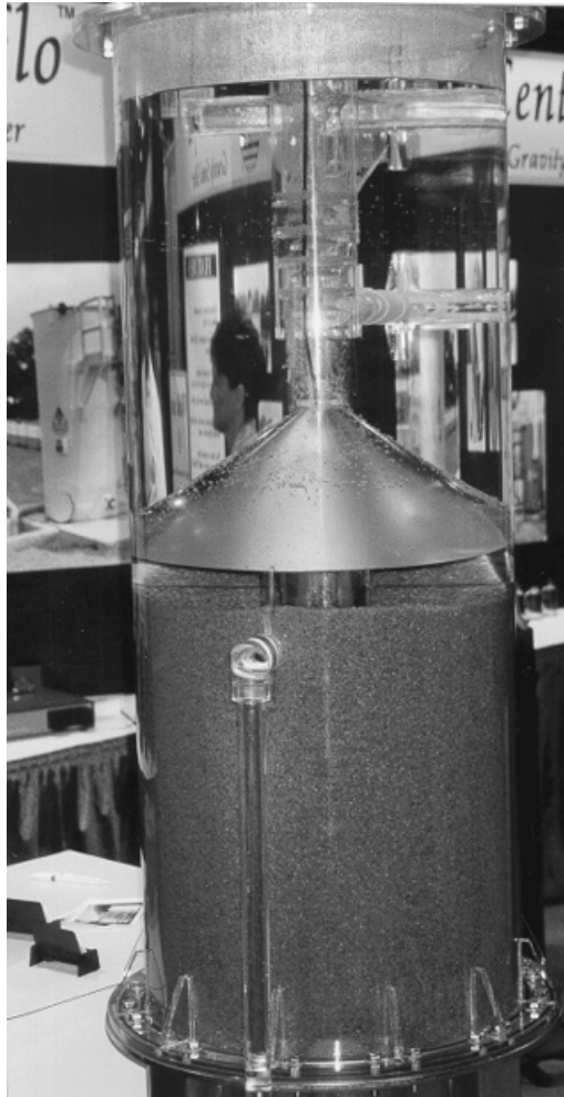
FIGURE 8.6 One view of a self cleaning sand filter.
