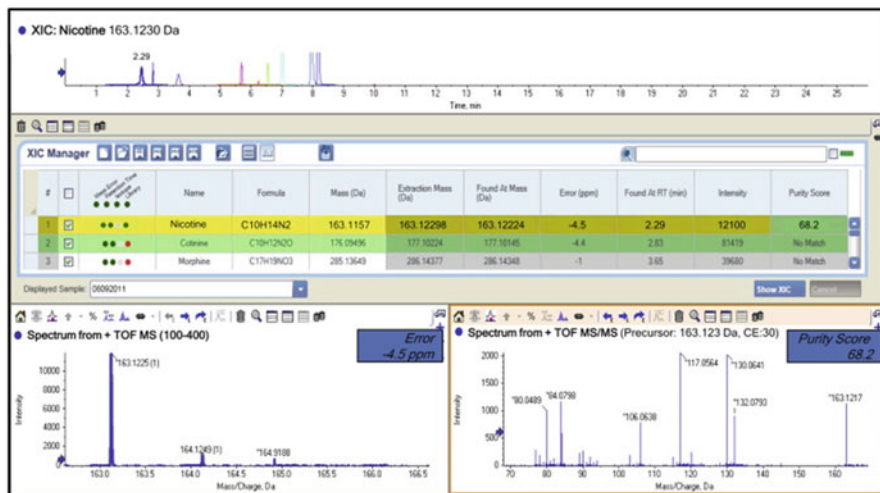
Fig. 1 Example of identification of the targeted compound nicotine in a river water sample based on accurate mass MS and MS/MS information (from Panditi et al. [46])
