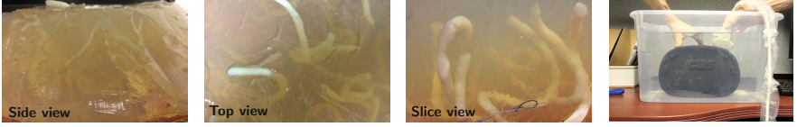
Fig. 2. Illustration of the noodle phantom , made of gelatine and Soba noodles (left three images) and an abdominal CIRS phantom mounted in a water tank (right)
