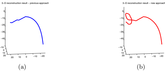
Fig. 7. Reconstruction result using the previous approach (a) and our new method (b). While both methods perform well for the linear part of the catheter, the previous approach fails for the curved catheter tip.
