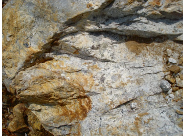
Photo 9.2 Mo-Cu mineralization occurred at well-developed quartzitization and K-feldsparization areas; O Quy Ho site
