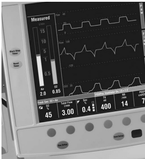
FIGURE 15-14 Electronic control of inspired oxygen, carrier gas, and total fresh gas flow, Aisys. (Courtesy GE Healthcare, Madison, Wis.)
