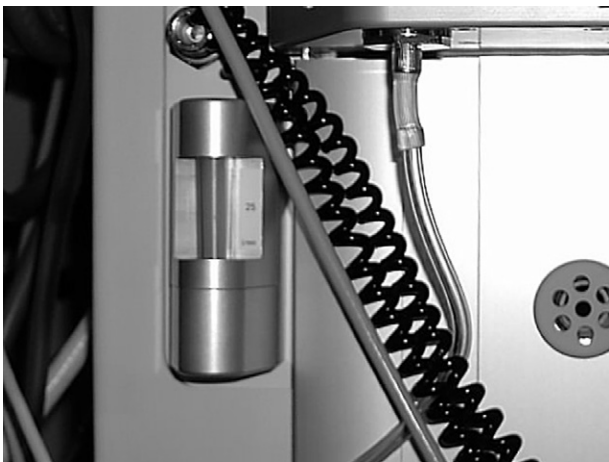
FIGURE 15-21 The scavenger suction flowmeter on the ADU is located behind and beneath the bellows block on the left side of the machine.
