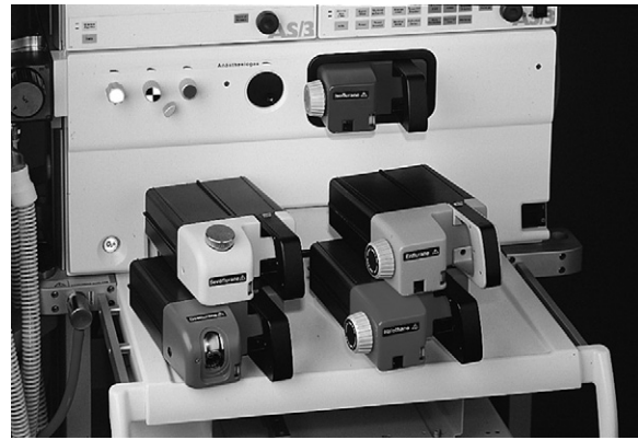
FIGURE 15-33 Datex-Ohmeda ADU vaporizer cassettes. The isoflurane cassette is plugged into the vaporizer port, and controls may be adjusted with the control wheel to the left of the port. (Courtesy Datex-Ohmeda, Tewksbury, Mass.)
