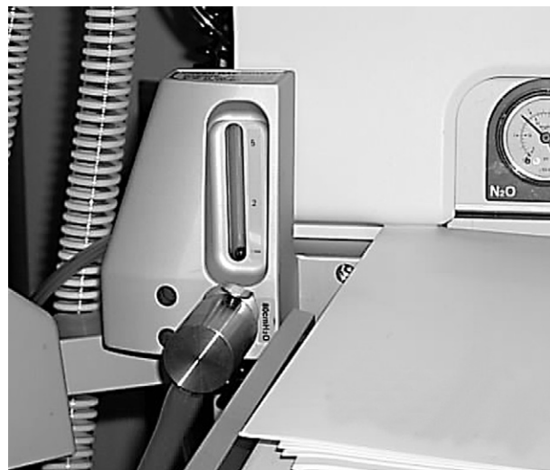
FIGURE 15-20 The common gas outlet flowmeter on the ADU is located to the left of the writing surface. (From S/5 Anesthesia Delivery Unit User's Reference Manual , Catalog No. 8502304. Madison, Wis: Datex-Ohmeda; 2000.)
