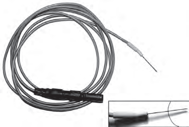
Fig. 8: Subdermal needle electrode: 1 cm steel electrodes used for EEG, EP and AMAP
