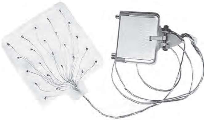
Fig. 3: Silver/silver chloride plate array of 25 electrodes (5 × 5 cm). These are used for corticograms to localise central sulcus or epileptic foci
