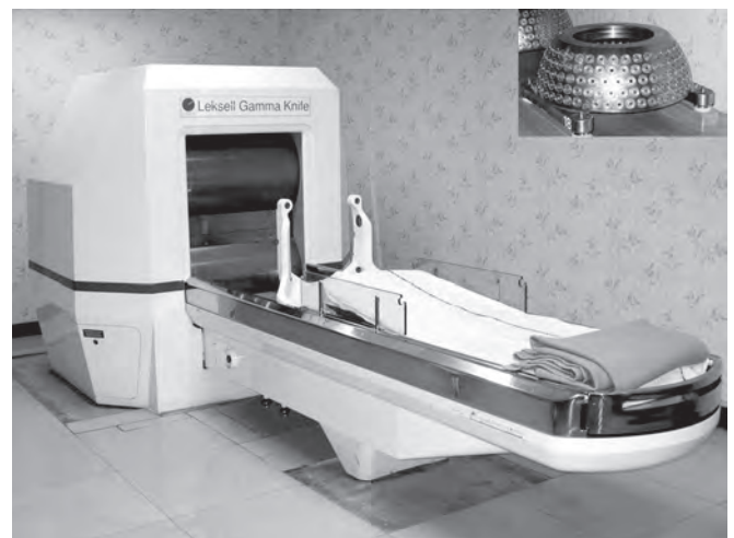
Fig. 4: The Leksell Gamma Knife Unit B. The collimators are seen in the inset
