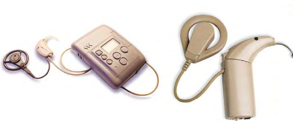
Fig. 41: External components of auditory brainstem implant
