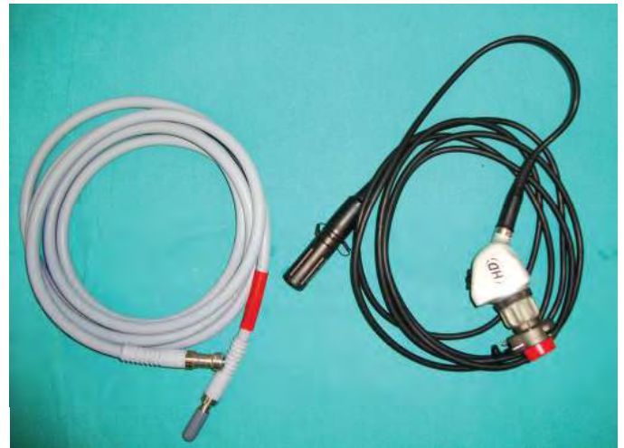
Fig. 29: Light source and camera for endoscope
