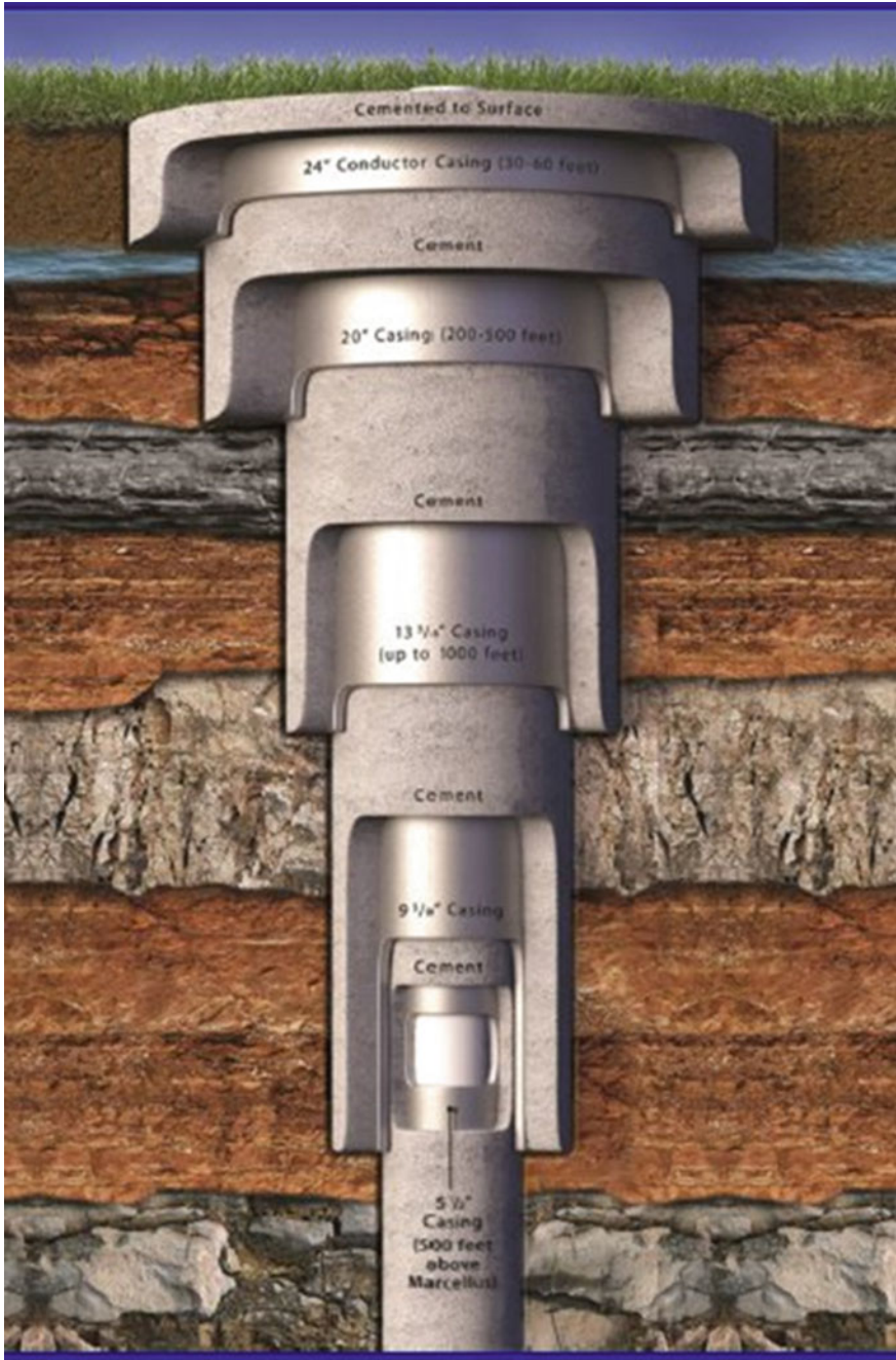
Fig. 2.3 Casing program in the Marcellus area [Source Frantz (2014)]. The vertical scale has been greatly compressed, as oil wells are typically more than 1500 m (5000 ft) deep
