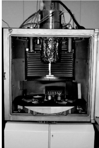
Fig. 7.9. Interior of APS 1100 IAD deposition system (Courtesy of Leybold Optics, Alzenau, Germany)
