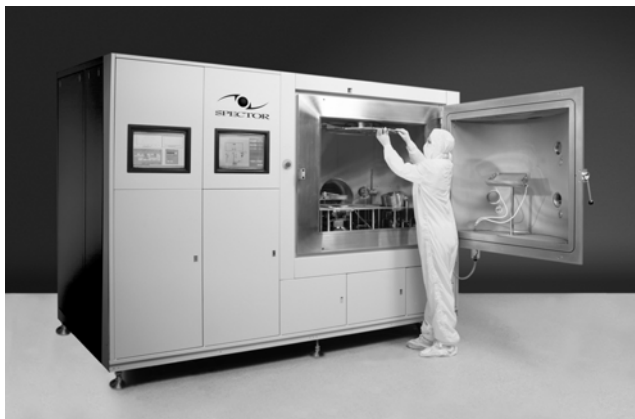
Fig. 7.10. SPECTOR DIBS deposition system (Courtesy of Veeco Instruments Inc., Woodbury, NY, US)
