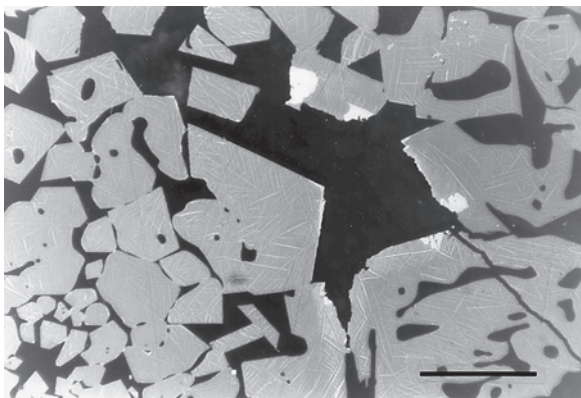
Fig. 6.33. Faynan 1, sample JD-1/33a. Idiomorphic crystals consisting of crednerite (filling) and Cu-bixbyite (lamellae, rim, and inclusions) at the rim of a gas bubble. The crystals were most likely formed through the reduction of Cu-Mn ores (scale 0.1 mm; reflected light, oil immersion)
