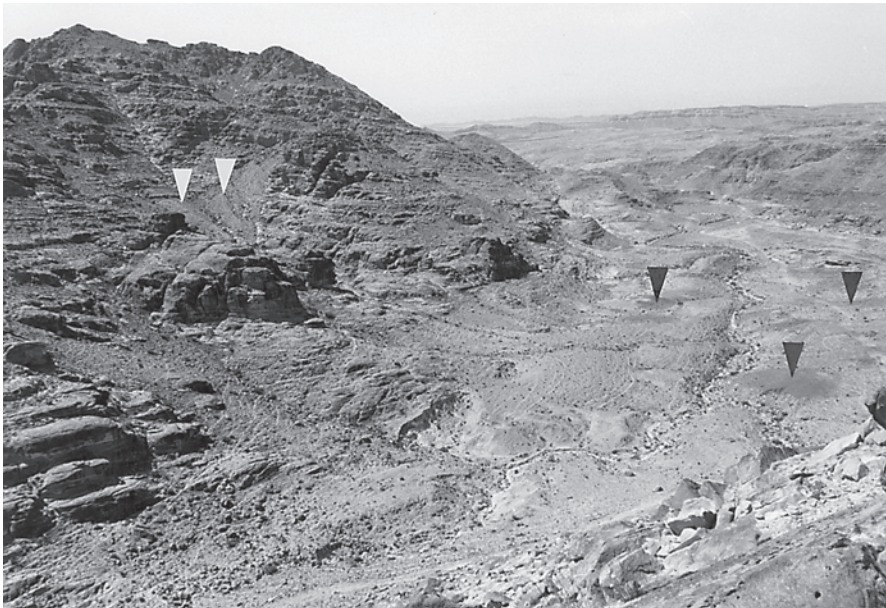
Fig. 5.22. The mining district of Wadi Abiad. At the bottom of the valley, Iron Age mining can be observed, exploiting the ore mineralizations of the DLS ( dark arrows ), which were not exposed to the surface. The waste dumps to the left of the photo ( white arrows ) date back to the Roman period and are evidence of mining into the MBS (from Heitkemper 1988)
