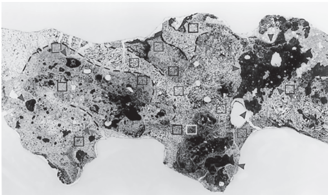
Fig. 6.4. Wadi Fidan 4, sample JD-8/24. Section through an Early Bronze Age I Ca-Mg silicate slag with a low degree of liquefaction. One can recognize the partly decomposed (sandy) dolomites ( marked areas ); in between are crystallized areas and dispersed inclusions of cuprite ( arrows ). Those sections, whose chemical compositions have been measured with EDS, are marked (see Table A.5) (width of piece: 3.7 cm)
