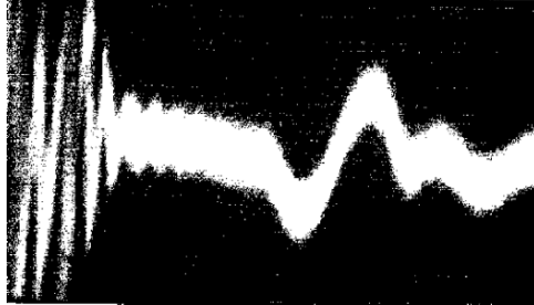
Fig. 19.13. “DC”-acoustic compression pulses observed for glass-YZ-LiNbO 3 interface driven by 15-MHz acoustic excitation.
