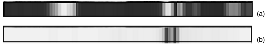
Fig. 29.5. Defect selective imaging with air-coupled ultrasound: fundamental frequency (a) and wave modulation (b) B-scans of the area with linear (drop of water, left) and nonlinear (crack, right) defects.
