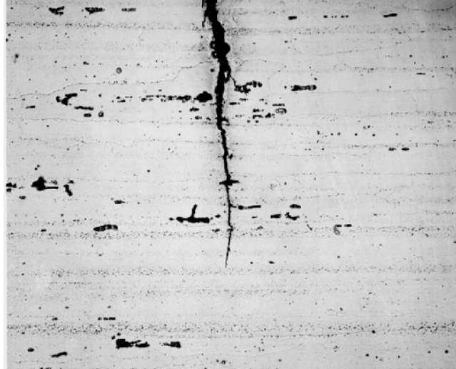
Fig. 31.2. Fatigue crack in Aluminum AA 7075.
