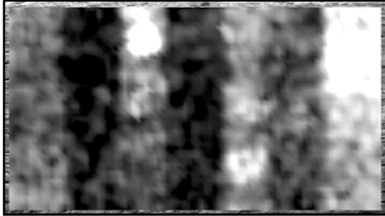
Fig. 29.3. Fourth-harmonic image of periodic delaminations between oak veneer lamina and particleboard plate. The specimen length is 12 cm.
