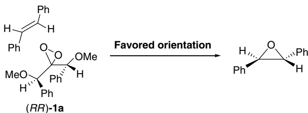
Fig. 8 Favored orientation in epoxidation of trans -stilbene by dioxirane (RR)-1a
