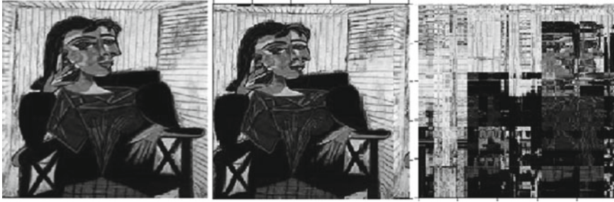
Fig. 19.11 Grayscaled to left, recovered by the edge method in the middle frame and attempted recovery using leaf ordering after Ward's Hierarchical Clustering in the frame to the right
