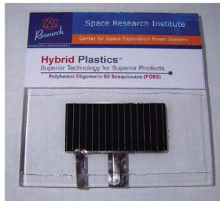
Fig. 8.25 Solar cell with POS conformal coating
