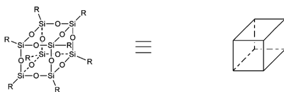
Fig. 4.1 Chemical structure and schematic representation of T_8 POS
