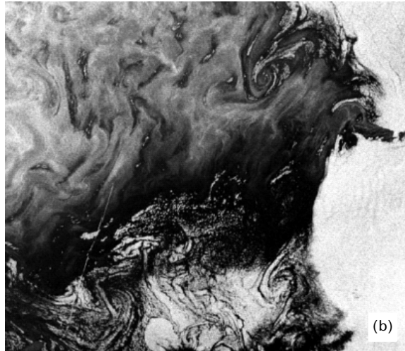
Figure 4.16. (a) Photo of typical grease ice observed in the ice edge region. (b) Sub-image of an ERS-1 SAR scene covering about 50 \times 50 km from the marginal ice zone, showing the characteristic signature of grease ice (dark), pancake floes (bright area in the upper left part of the image) and open water (almost white area on the right-hand side of the image generated by winds of 5\text{--}10\text{ m s}^{-1} ). The SAR image was obtained in the Barents Sea during the SIZEX experiment in March 1992 (Johannessen et al. , 2003).
