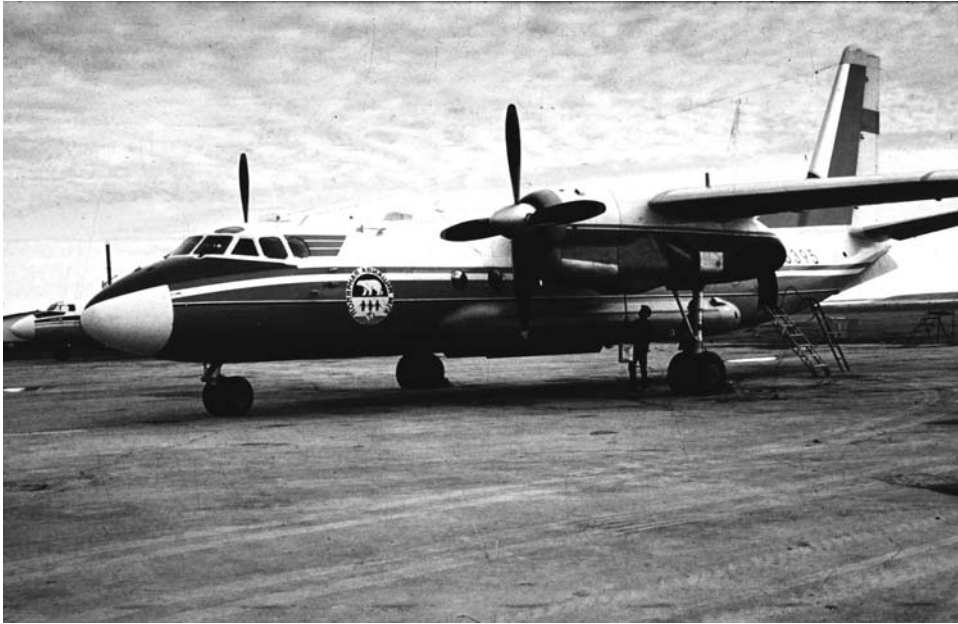
Figure 3.4. Ice reconnaissance aircraft AN-24T equipped with SLAR Toros.
