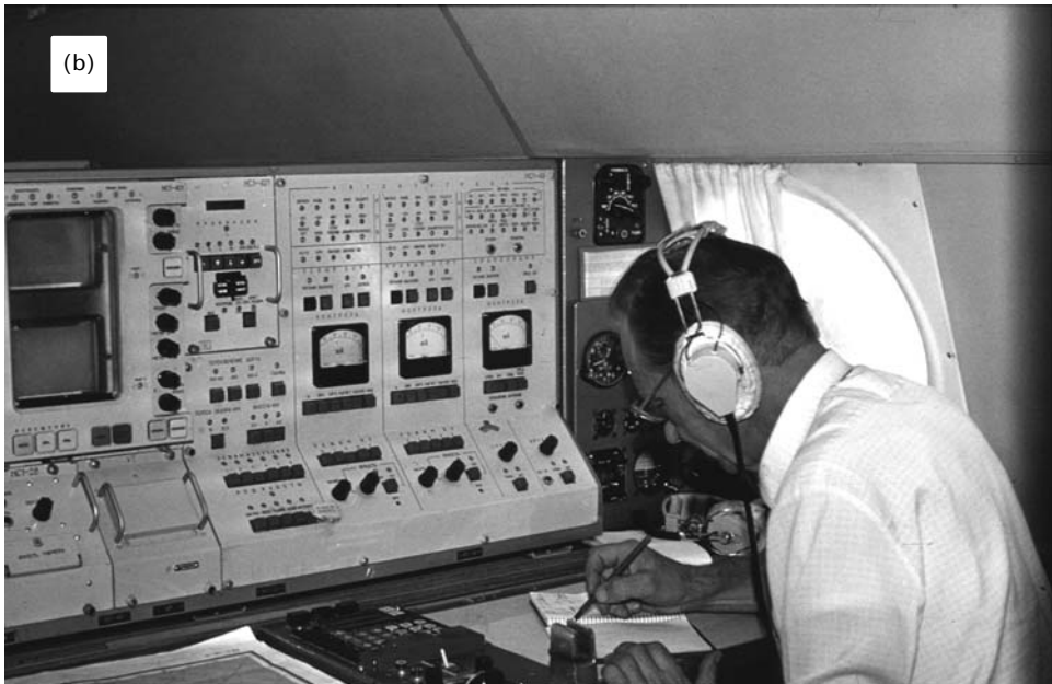
Figure 3.7. (a) Aircraft of remote ice reconnaissance IL-24N (base aircraft IL-18D ) equipped with the radar system Nit'-C; (b) Panel of on-line depiction of radar images and control of the Nit'-C system onboard IL-24N .
