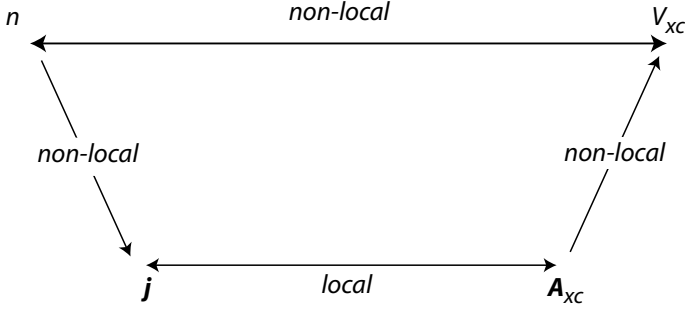
Fig. 5.1. Diagram showing the relation between current density functional theory and density functional theory. The nonlocal relation between n and v_{xc} is transformed into a local relation between \mathbf{j} and \mathbf{A}_{xc} by means of two non-local transformations from n to \mathbf{j} and from v_{xc} to \mathbf{A}_{xc}
