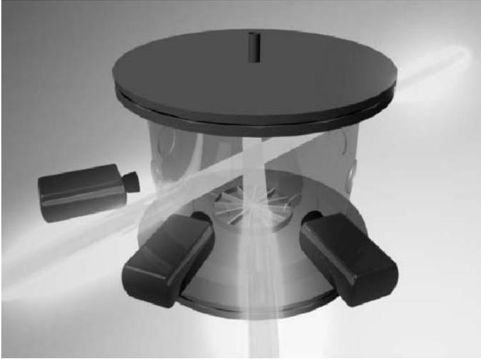
**Fig. 1.** A sketch of the flow apparatus, cameras and lasers.
