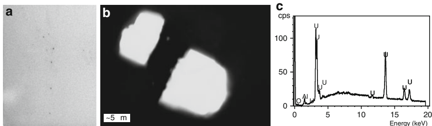
Fig. 8 Radioactive particles in Ravenglass estuary sediments (Lind 2006). (a) Digital autoradiography of Ravenglass surface sediments (0–5 cm). (b) Electron micrograph (BEI mode) of two particles with X-ray microanalysis (c) confirming the presence of U. Bar = 5 \mu\text{m} . The appearance of the particles indicates that they were actually one particle which was divided upon manipulation
