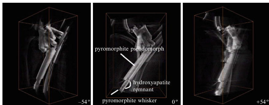
Fig. 10 An example of electron tomography. The images are the ones tilted at 0^\circ and \pm 54^\circ of BFTEM tomography. Hydroxypyromorphite nanocrystallite whisker and pseudomorph formed on hydroxyapatite are shown in three dimensions (Kamiishi and Utsunomiya, submitted). Full movie of BFTEM tomography is available on the web site ( http://mole.rc.kyushu-u.ac.jp/~ircl/ )
