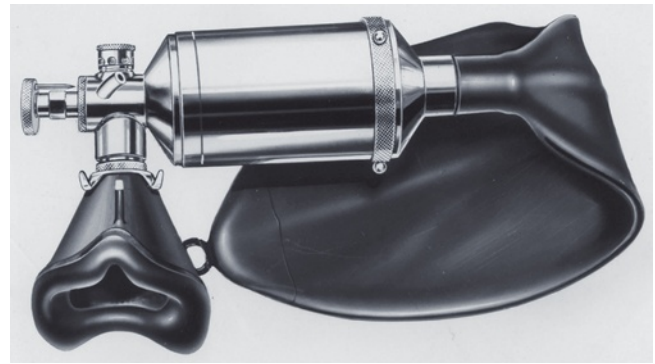
Fig. 52.10 In the to-and-fro system developed by Ralph Waters, the carbon dioxide absorbent was placed in the large canister. The patient breathed back and forth (to and from the reservoir bag attached to the distal end of the canister) through this valveless system. There were two problems with this elegantly simple system: 1) The absorbent at the proximal (patient) end of the canister exhausted first, increasing the dead space. 2) The absorbent tended to settle, resulting in a low resistance pathway at the top of the absorber
