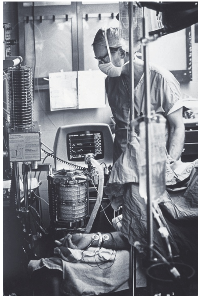
Fig. 55.3 Mass spectrometer anesthetic and respiratory gas analysis operating room display screen in Moffitt Hospital with author, 1978. (Courtesy of the author’s collection.)
