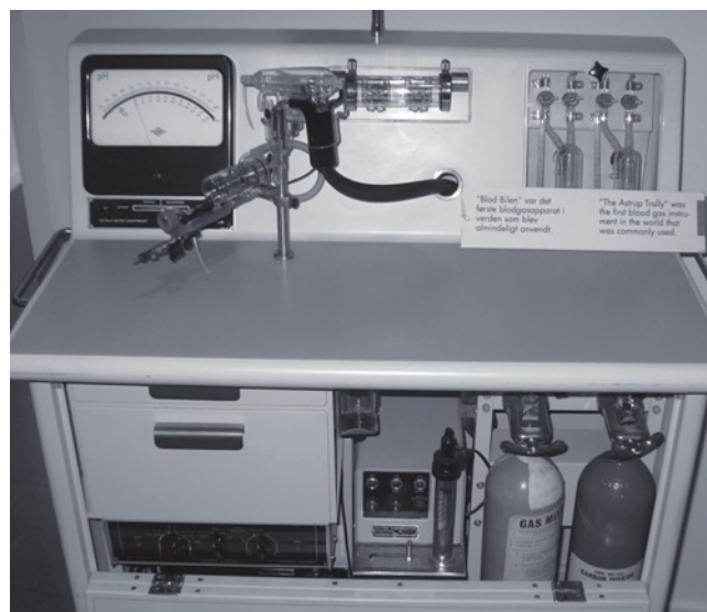
Fig. 55.8 Blood gas analyzer using the Astrup equilibration method for \text{PCO}_2 , with micro-capillary pH electrode and equilibrators designed by Siggaard Andersen, and the Clark electrode for \text{PO}_2 analysis. “S”: sampling tip on hand-held pH electrode, also used to connect pH sample to KCl reference electrode. (Radiometer Co, Copenhagen, ~1960). (Courtesy of the author’s collection.)
