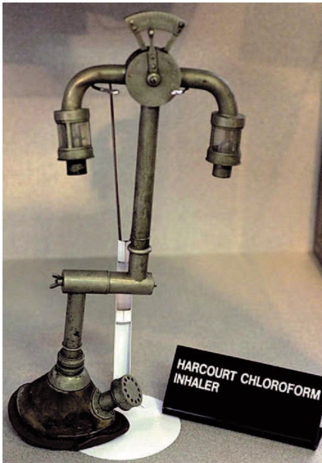
Fig. 53.3 The Harcourt vaporizer was designed to produce a known delivered concentration of chloroform. Two glass bulbs, probably long since broken, were attached to the two arms. The vaporizer compensated for the effect of the temperature of the chloroform on the concentration produced. (Courtesy of the Wood Library-Museum of Anesthesiology, Park Ridge, IL)
