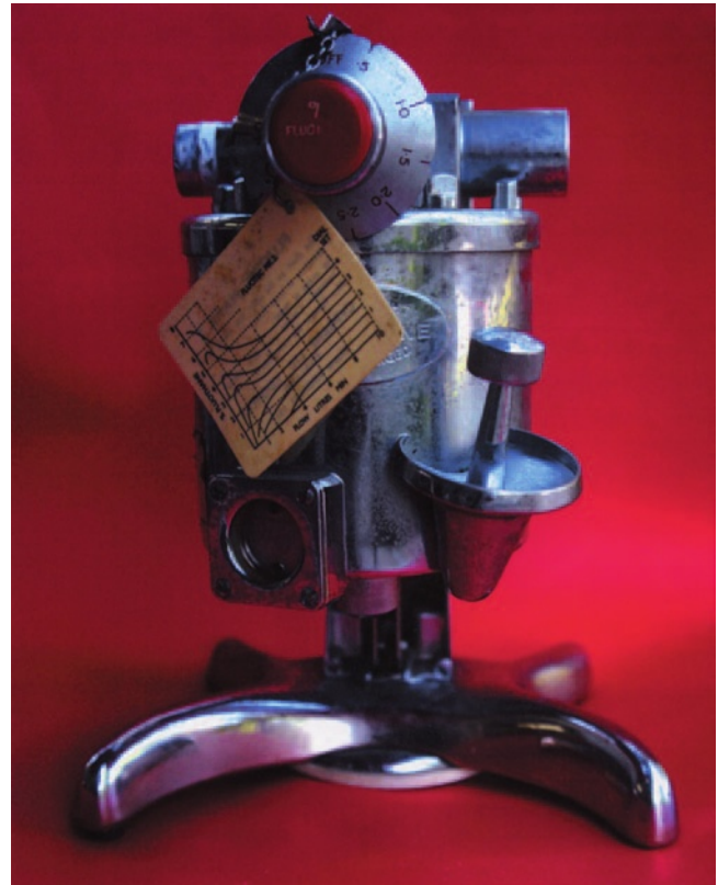
Fig. 52.9 Fluotec Mark II Vaporizer. Note the card chained to the vaporizer with a graph showing how fresh gas flow affected the vaporizer output. A predictable (flat line) output was accomplished at inflow rates of 1–2 l/min or more for this early model. Later versions produced constant known outputs at flows as low as a few 100 ml/min
