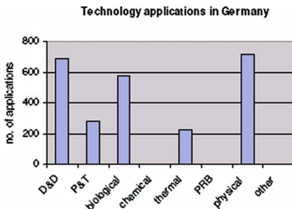
Fig. 6.2 Number of remedial technology applications in Germany (Spira 2006; RefAS 1995). D&D = Dig and Dump; P&T = Pump and Treat; PRB = Permeable Reactive Barrier
