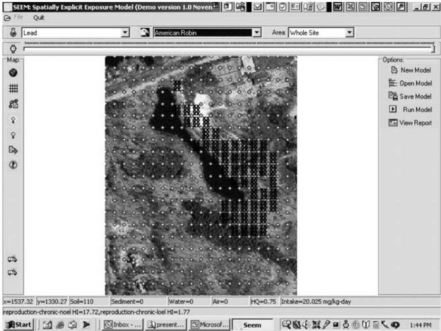
Fig. 4.3 User interface of SEEM. Imported map is aerial photography. Cross hatching indicates areas of highest modeled risk estimates from soil lead exposure to the American robin ( Turdus migratorius )
