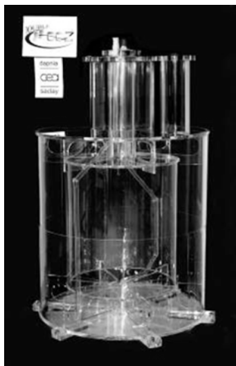
Figure 3. Double Vessel acrylic mockup, scale 1/5th of the Double Chooz detector.
