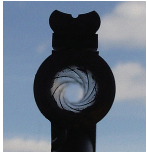
Figure 11.18. Photograph through the barrel of a rifle barrel showing the spiral rifling needed to cause a dart to spin on its horizontal axis during flight.
