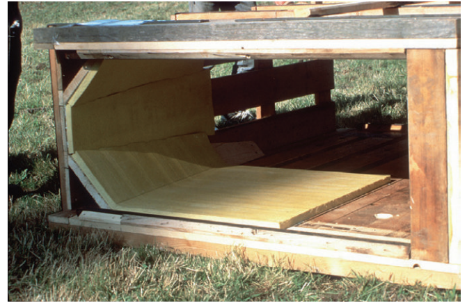
Figure 52.3. Head and neck movement in transport crates is restricted with padding in order to reduce the risk of a horse turning onto its back at take off during air transport.
