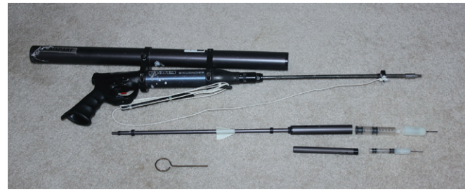
Figure 16.8. An underwater dart system with laser apparatus (AQUADART, Harvey et al. 1988).
