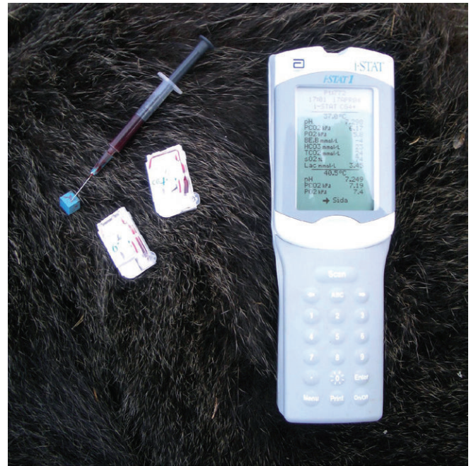
Figure 5.3. The i-STAT ® 1 Portable Clinical Analyzer and cartridges used for field analysis.
