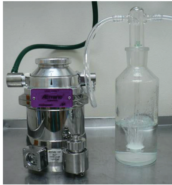
Figure 27.5. In-line bubbler bottle for humidification of transport and anesthetic gases.
