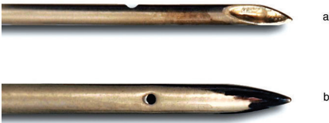
Figure 11.7. Photograph of two needle types used in two types of two-chambered compressed gas darts. (a) A hypodermic needle that has the sharp tip occluded with solder used in blow darts. (b) A thicker, blunter, machined needle used in molded nylon darts.
