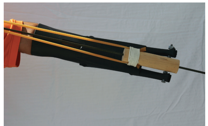
Figure 15.12. An example of a Hawaiian sling. It is recommended that this only be used for long distances with skilled users or for euthanasia purposes due the power of the propulsion of the tip.
