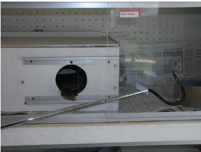
Figure 20.7. Shift box in cage. Shift box door can be slid close with a snake hook and locked. Black mamba, Dendroaspis polylepis (courtesy of Medtoxin Venom Laboratories).
