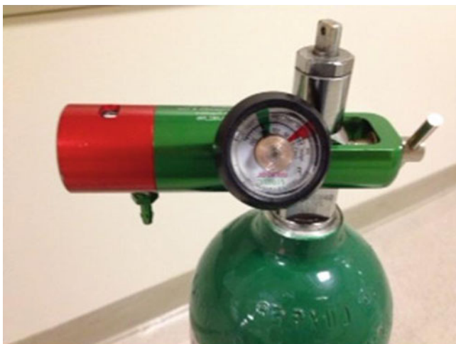
Fig. 6.4 Oxygen tank with detachable regulator and flow control knob (red)
