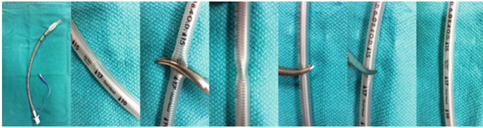
Fig. 15.5 A hemostat is used to simulate a patient biting on an anode tube. Note that the tube is not completely occluded and can be reformed using a hemostat
