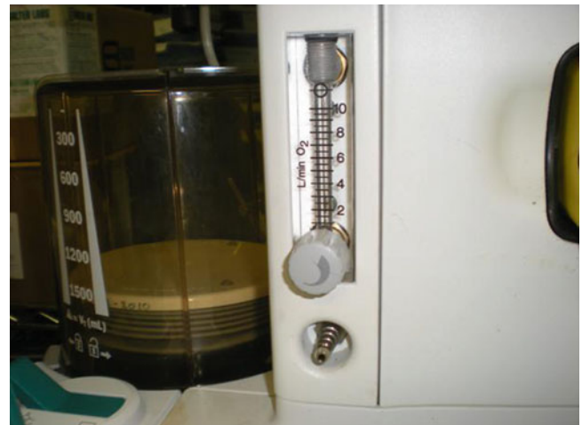
Fig. 6.22 Auxiliary oxygen flow meter (0–10 L/min) and outlet nipple
