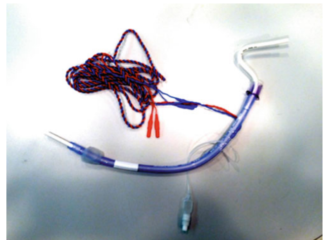
Fig. 14.9 Surface-embedded electrode endotracheal tube with an intubating stylette to improve intubation success
