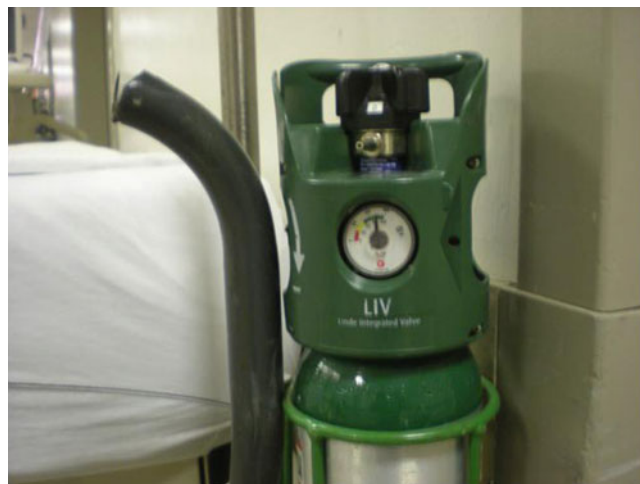
Fig. 6.5 Oxygen cylinder with integrated reducing valve and flow control for flows of 0.25–25 L/min
