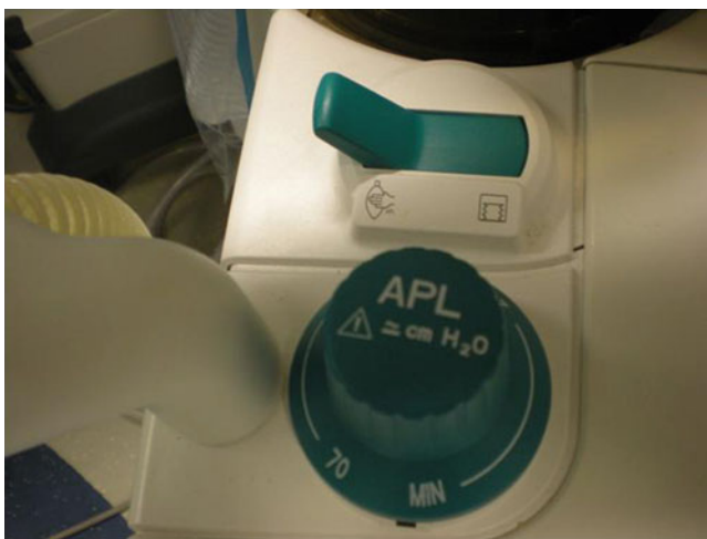
Fig. 6.26 Adjustable pressure-limiting (APL or “pop-off”) valve and bag/ventilator selector switch
