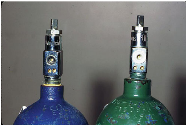
Fig. 6.10 Pin-indexed safety system for medical gas cylinders. Nitrous (blue) and oxygen (green) tanks showing different positions of the receptacles where the two pins in the hanger yokes would engage for each of these two gases. This system is a national standard
