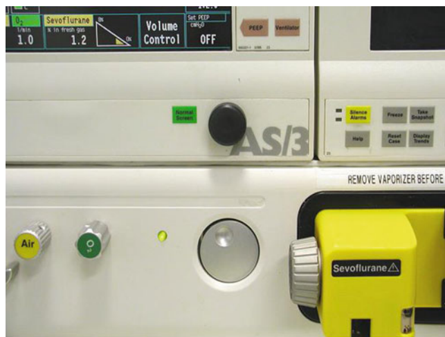
Fig. 6.20 Aladin electronic vaporizing system on GE Datex ADU workstation. The yellow cartridge is agent-specific for sevoflurane. In the ADU the large silver colored wheel controls agent concentration and is rotated clockwise to decrease concentration. Clearly (from Figs. 6.18, 6.19 and this figure) it is important to know in which direction to turn the wheel/dial to change agent concentration so as to avoid an unintended overdose or underdose
