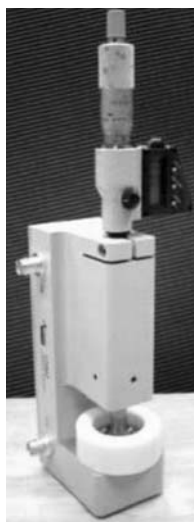
Fig. 4.16. Capacitor cell. The capacitor had stainless steel plates 20 mm diameter, with a precision digital micrometer controlling the plate separation (to 3\ \mu\text{m} precision), and a Teflon sample holder. Sample volume was \sim 1\ \text{mL}
