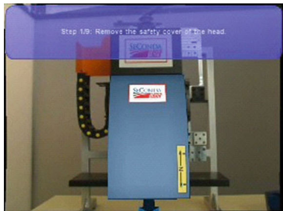
Fig. 13.9 AR view of the remote maintenance application with text and 3D virtual data
