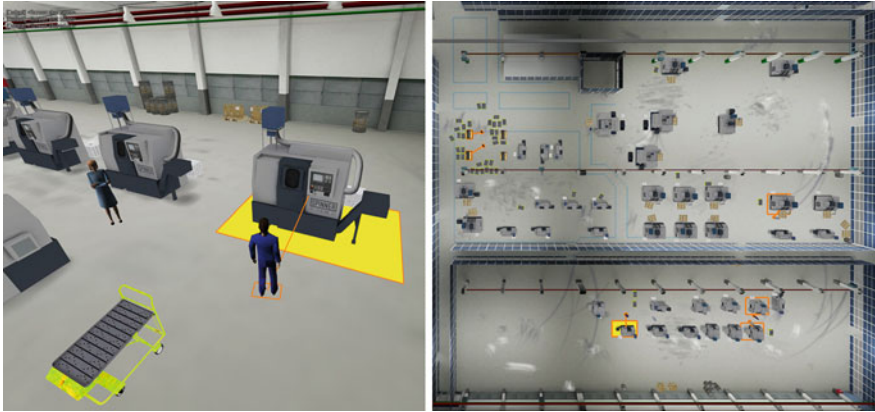
Fig. 12.5 Two different views on the factory layout: walking inside the virtual factory ( left ) and the top view ( right ) with the roof automatically hidden
