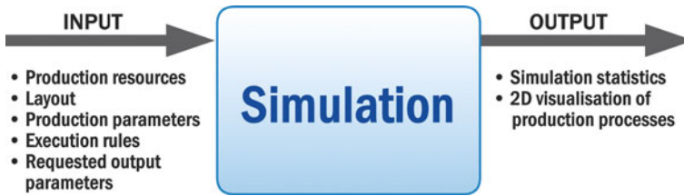
Fig. 14.4 The input and output of the simulation module
