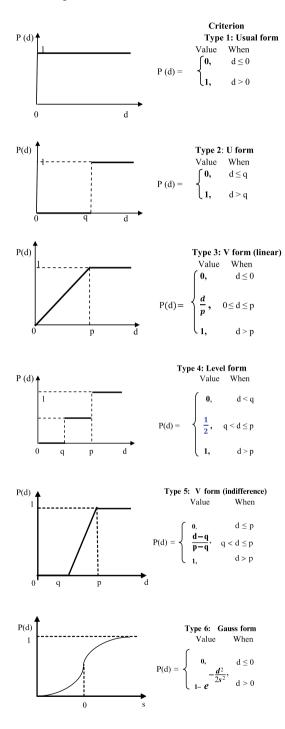
Fig. 3.3 Transfer functions
