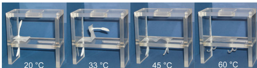
Fig. 8 Triple-shape effect of a multiphase polymer network with poly( \epsilon -caprolactone) network chains and poly(ethylene glycol) side chains. The picture series shows the recovery of shapes B and C by subsequent heating from 20 to 60°C, beginning from shape A, which was obtained as a result of the two-step triple-shape creation process. The object consisting of a plate with anchors demonstrates a fastener device
