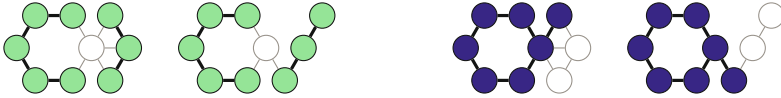
Fig. 1. A maximum common induced subgraph of the first two graphs has eight vertices, shaded. However, if we require the common subgraph to be connected, only seven vertices may be selected—one way to do this is shown in the third and fourth graphs.
