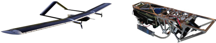
Fig. 4. (a) The senseSoar solar-powered UAV, developed at ETH Zurich. (b) Modular sensor pod for onboard processing and visual-inertial sensing.
