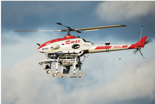
Fig. 5. The RMAX helicopter platform with the avionics box attached below the platform and the laser scanner facing downward mounted on a vibration isolated support placed under the helicopter nose. The color and thermal video cameras are mounted on a pan/tilt unit below the avionic box. The GNSS antenna is mounted on the helicopter tail boom.
