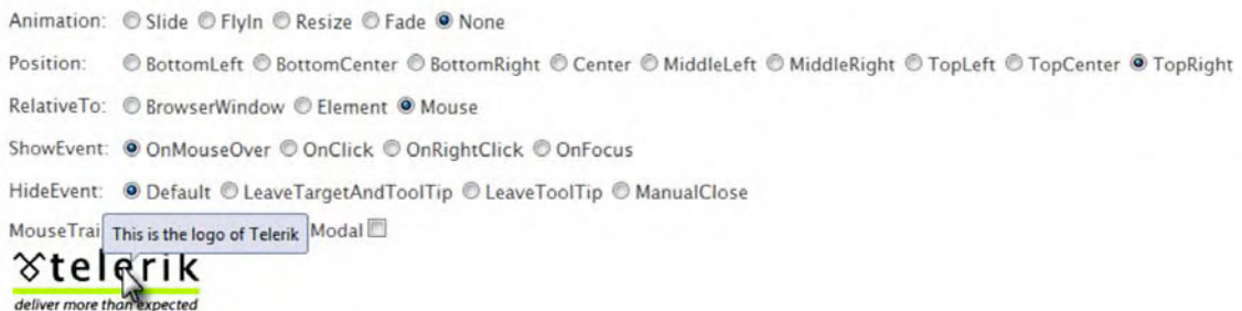
Figure 10-12. The RelativeTo property is set to Mouse and the Position property to TopRight . The RadToolTip is shown next to the mouse cursor.
