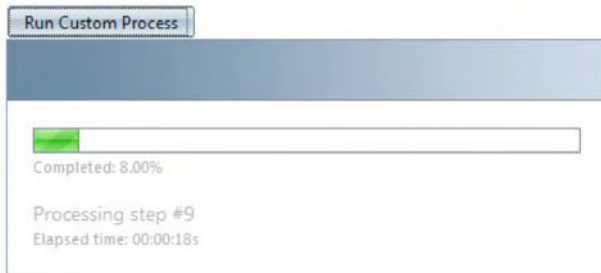
Figure 10-22. The process feeds information to RadProgressArea to display to users.
