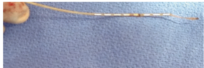
Fig. 38.4 Defected spinal cord stimulator lead. Contact number 4 with charring and different color; when on, patient felt electric shock in the mid-thoracic area. Photo courtesy of the University of Chicago Medicine, Department of Anesthesia and Critical Care
