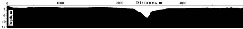
Figure 6.2. Bottom relief section across the strait connecting the eastern and western basins of the Large Aral Sea, from the Kulandy Peninsula. Note the deep channel in the central part of otherwise shallow strait.
