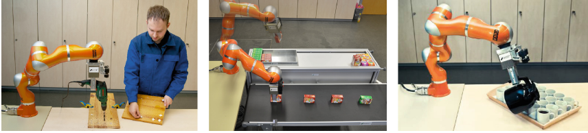
Fig. 1. Typical applications in SMEs or private households which require the execution of sensor based motions. From left to right: Drilling, Paletting, Pouring.
