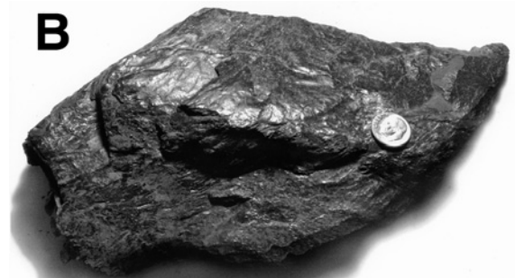
Fig. 6.10. Slickensides in a soft Cretaceous mudstone core, offshore Brazil (Courtesy of PETROBRAS), and from a mudstone in a fault along Pine Mountain in eastern Kentucky
