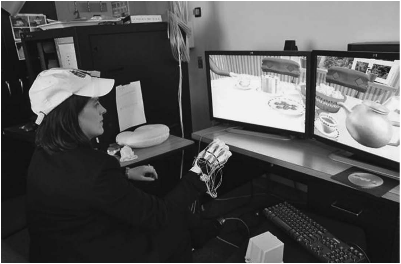
Figure 16.18 Virtual reality (VR) system assisting poststroke hand rehabilitation. The user wears a custom pneumatic glove, which assists finger extension. Magnetic trackers provide information regarding head orientation and hand location; the virtual scene is updated accordingly. Reproduced with permission from D. Tsoupikova, Electronic Visualization Laboratory. A color version of this figure can be found in Plate section 2.
