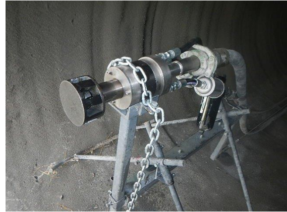
Figure 10. Liner casting head.
