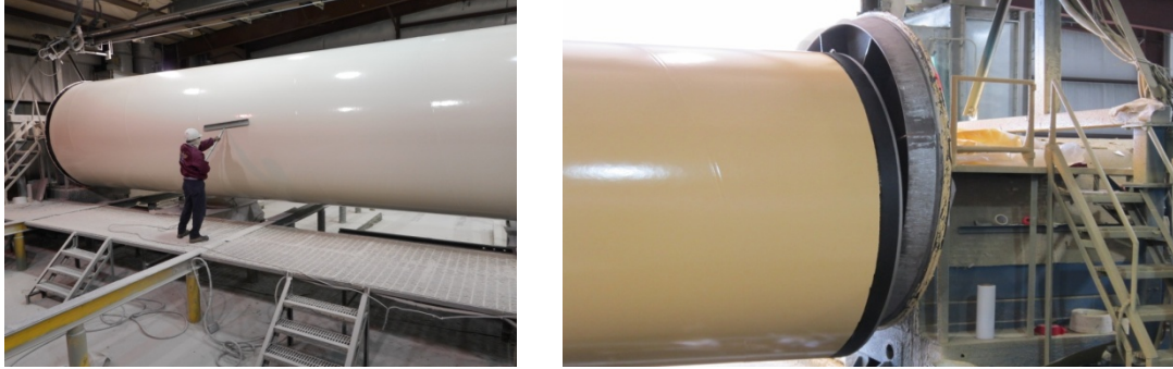
Figure 9a, b: Holiday Testing, Coated Pipe Just Off the Lathe
