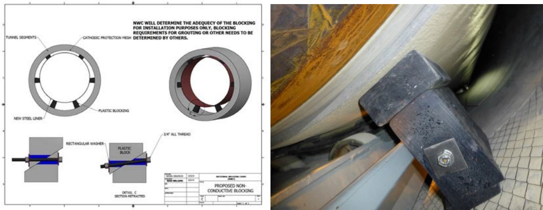
Figure 4a and b HDPE Adjustable Pipe Blocking System
