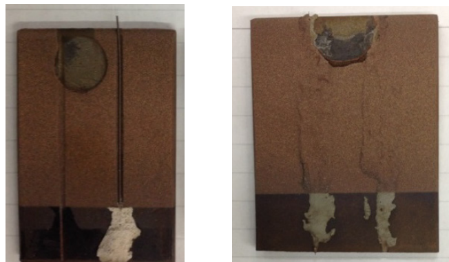
(a) High temperature Minco Epoxy (b) stainless-steel-based adhesive Figure 6. Sample condition after coating deposition
