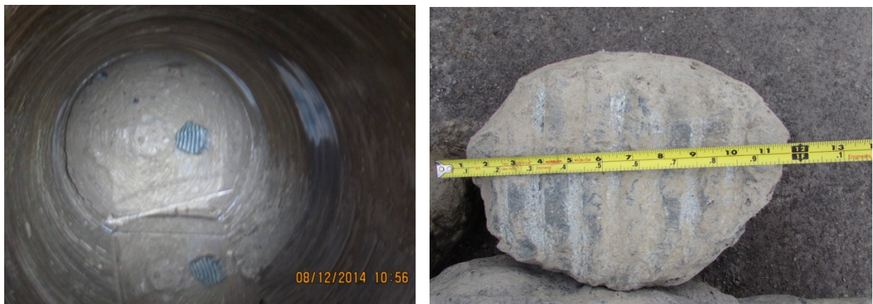
Figure 6. Cobble encountered during auger boring
