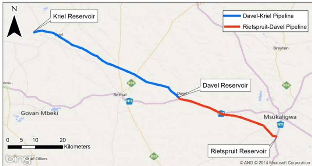
Figure 1: Alignment of the Rietspruit-Davel and Davel-Kriel Pipelines
