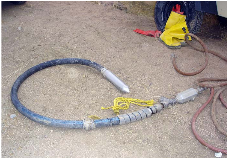
Figure 2 Internal Vibrator Used on Denver Water Board Project
