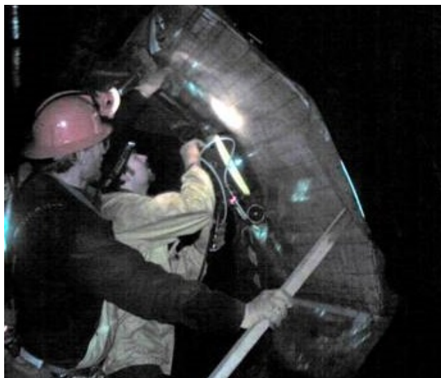
Figure 6. The 1 GHz hand held antenna that was used in the project.
