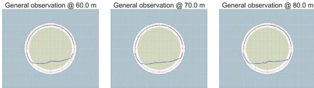
Figure 3. Showing an example of pipe cross-sections from the Huntingdon Trunk Sewer. The line represents sediment level in the pipe. This section had an average cross-sectional restriction of 9.0%.
