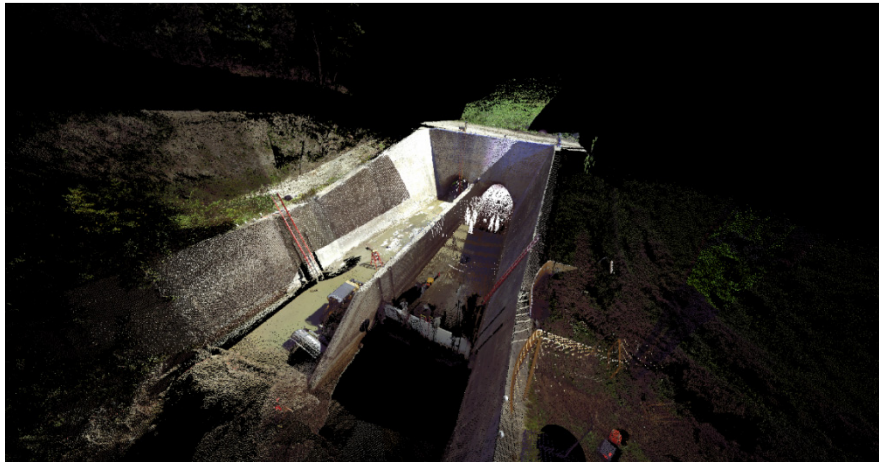
Figure 2. Colored point cloud model developed from 3D LiDAR laser data
