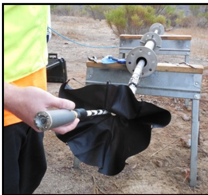
Figure 12. Left: Sensor head and drogue. Right: General setup for inspection.
