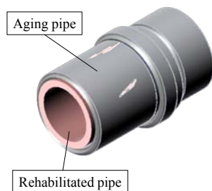
Figure 1. Pipeline after rehabilitation method has been performed.
