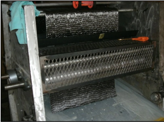
Figure 8 – CFRP Impregnating Machine
