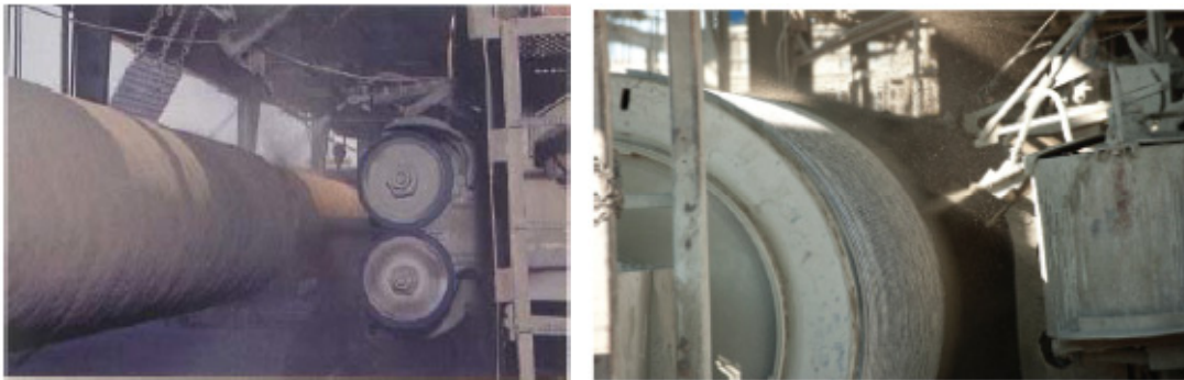
Figure 9 – Cement Mortar Coating
