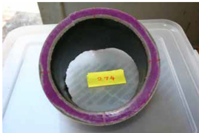
Figure 3: Cross Section of Phenolphthalein-Stained Pipe (Hu 2013a)
