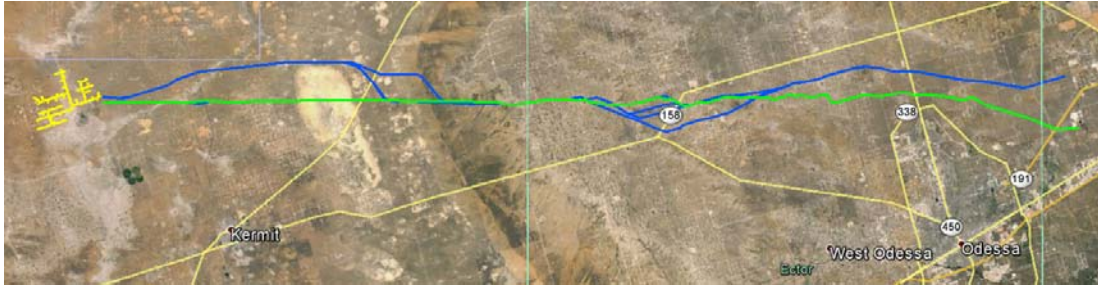
Figure 5. Rerouted Pipeline Alignment Versus Original Alignment
