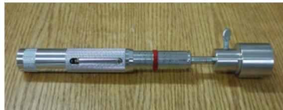
Figure 10: A pocket penetrometer can be used to determine CLSM strength prior to backfill.
