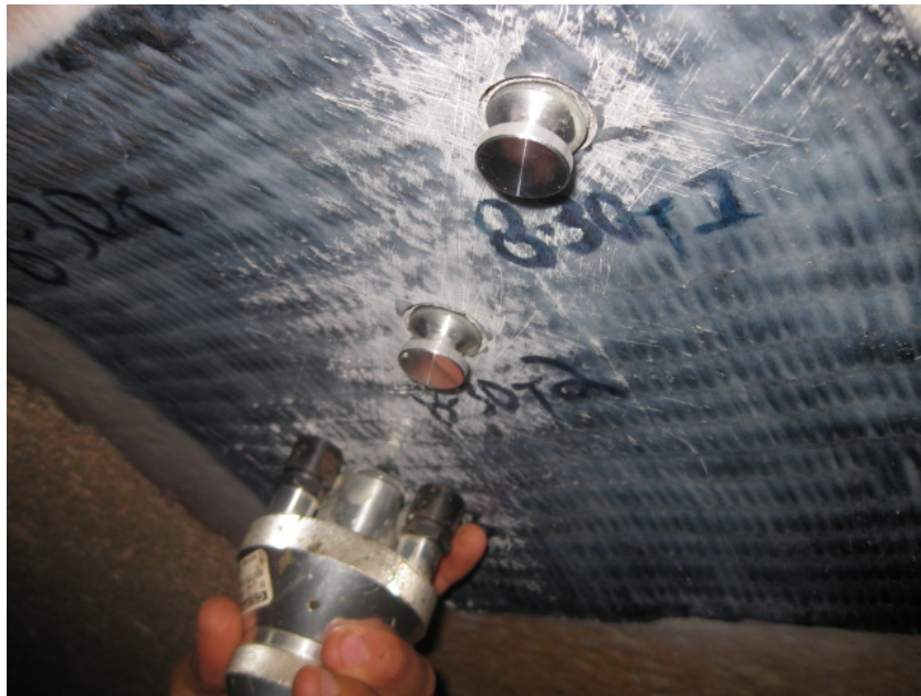
Figure 5. Pull Test per ASTM D4541
