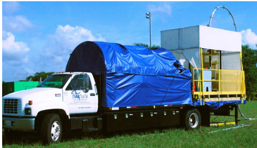
Figure 4 – Truck mounted unit for Hybrid FRP System steel reinforcement installation
