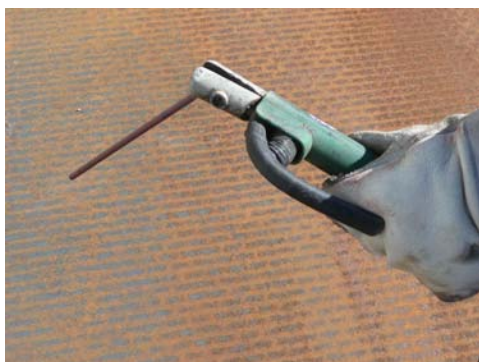
Figure 5a and b SMAW (Stick Welding) and FCAW (Flux Cored Arc Welding)
