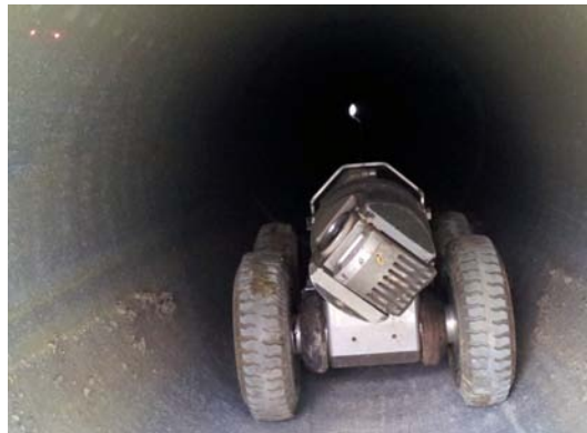
Figure 4. CCTV – Rotational laser diodes camera (from Rausch USA)
