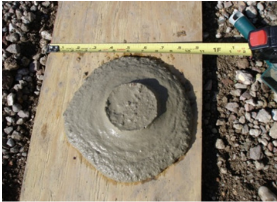
Figure 9: Measuring the spread diameter to determine flowability prior to placement.
