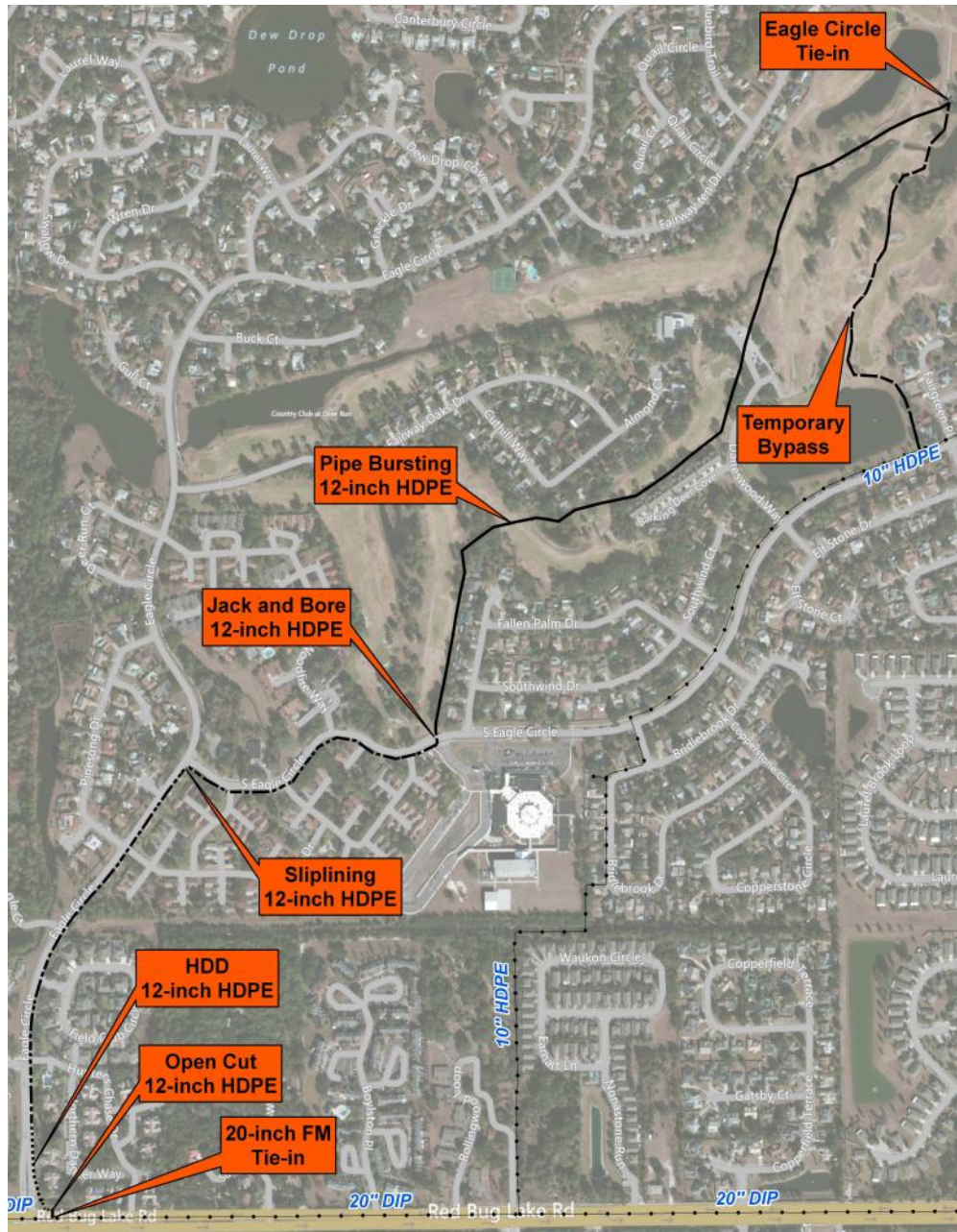
Figure 3. Replacement Pipe Installation Methods (Microsoft)
