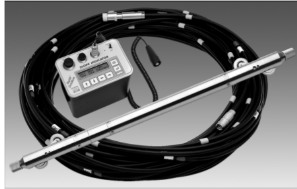
Figure 3. Horizontal Inclinometer Data Collection System (DGSI, 2013)
