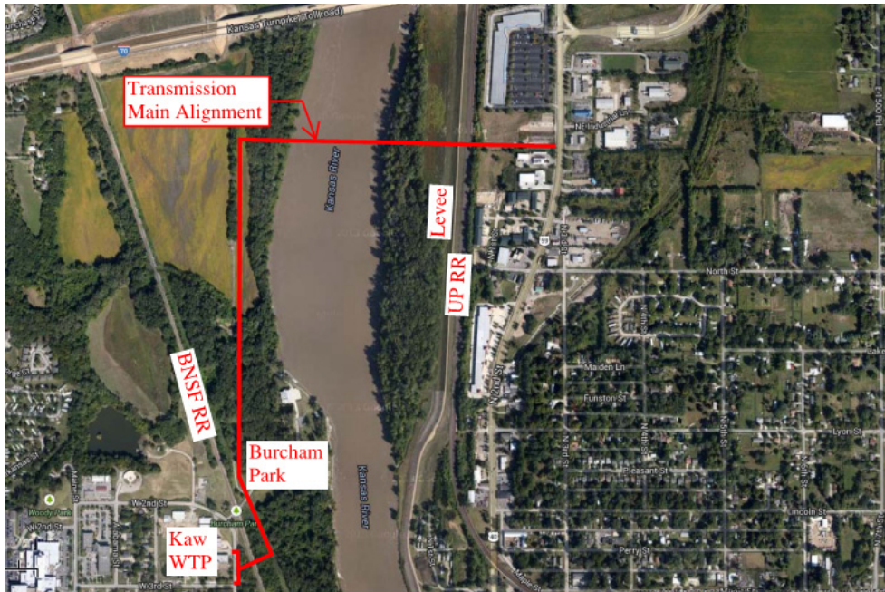
Figure 2 –Water Transmission Main Alignment
