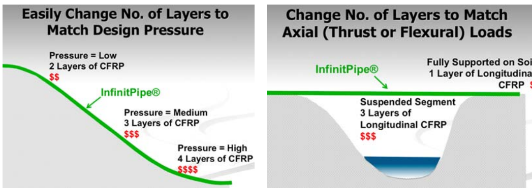
Figure 9. Design of onsite-manufactured pipe can be easily changed to accommodate changes in stresses along the pipeline.
