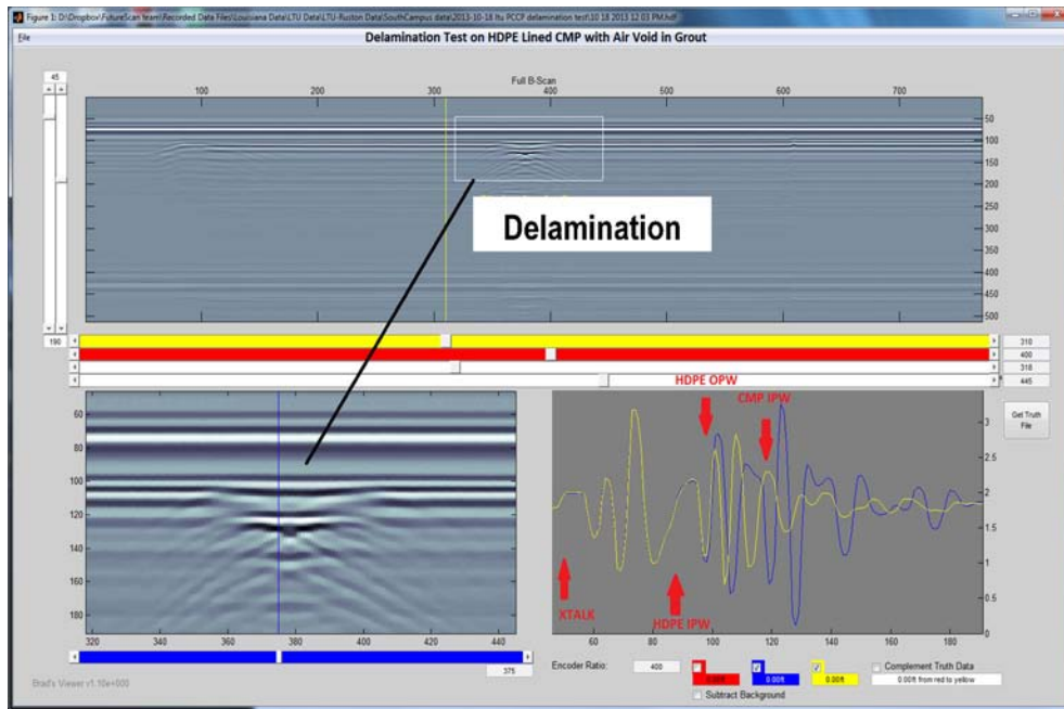
Figure 5: Screenshot from radar analysis: (top) 2D B-scan image of the pipe’s vertical cross-section near crown along its entire length; (left bottom) zoomed in window showing delamination; (right bottom) A-scan waveforms (signal strength vs. time delay) showing interfaces between HDPE, grout and the metal pipe.
