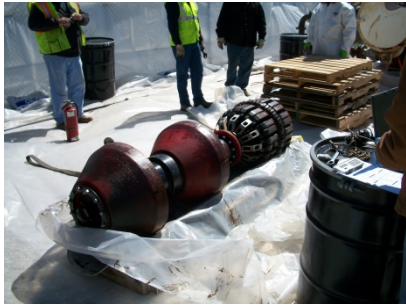
Figure 17 MFL Tool Extracted from Receiver
