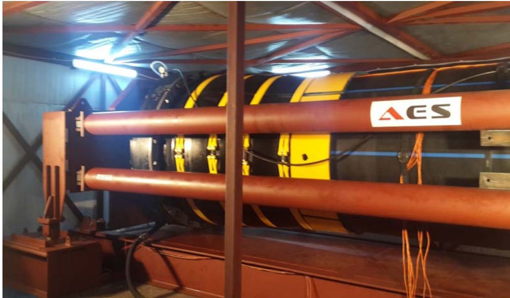
Figure 10: Test for the Whole Flange Connection
