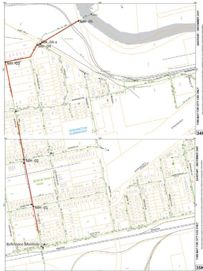
Figure 3. Location of the Del Norte Trunk Sewer, Stockton, CA. Inspected segments are marked in red.
