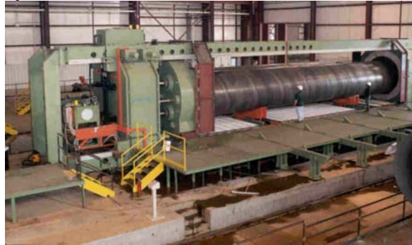
Figure 6 – Shop Hydrostatic Testing
