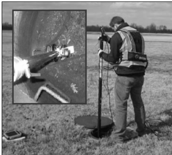
Figure 3. A technician operating the pole camera during a pipe inspection
