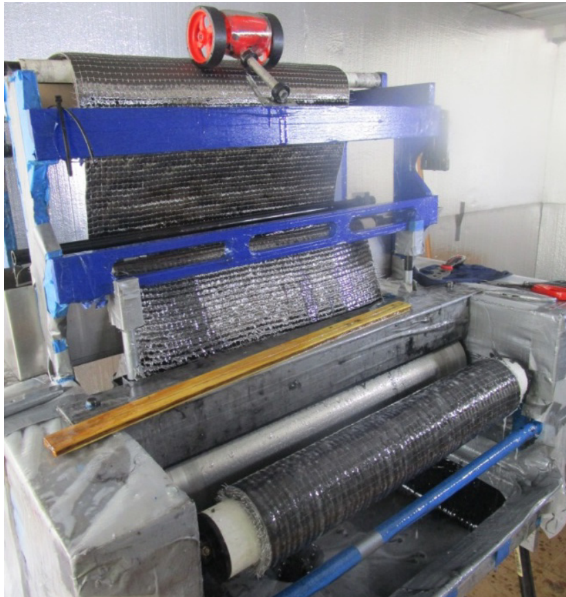
Figure 7. Mechanical saturation of the carbon fiber fabric.
