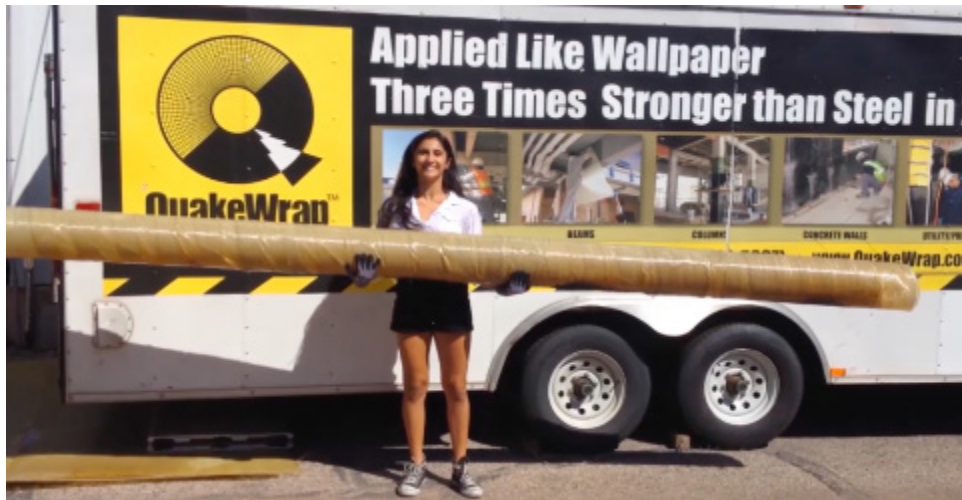
Figure 8. First sample of onsite-manufactured pipe is very light and easy to handle.
