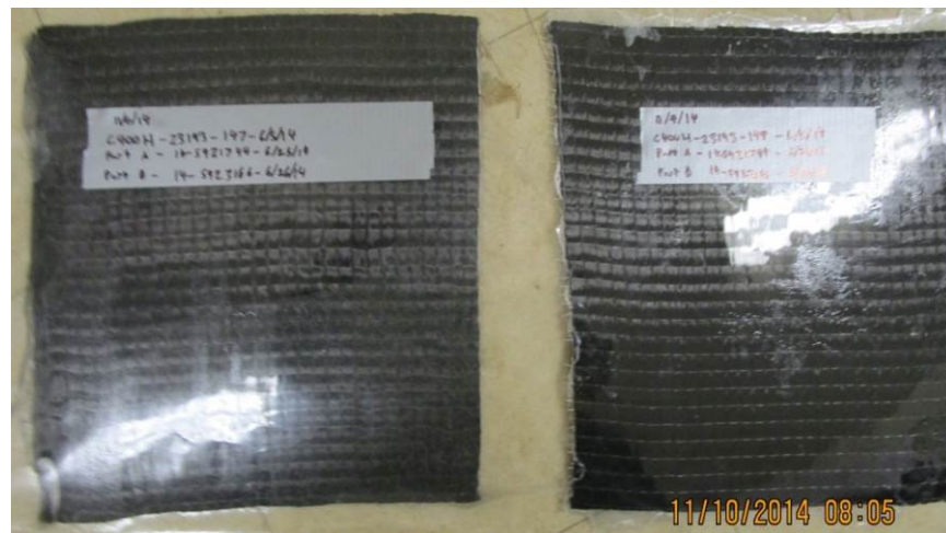
Figure 2. Witness panels utilized to confirm material design values.
