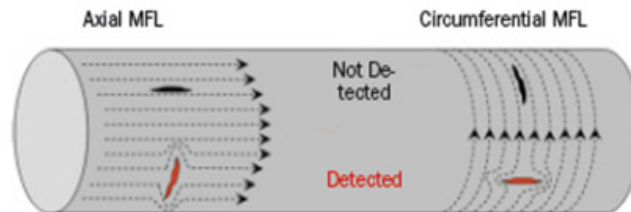
Figure 4 Solid (MFL) Figure 5 Anomalies detected by axial and circumferential flux lines
