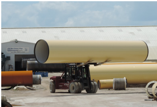
Figure 14: 108" pipe on padded forks in manufacturing facility
