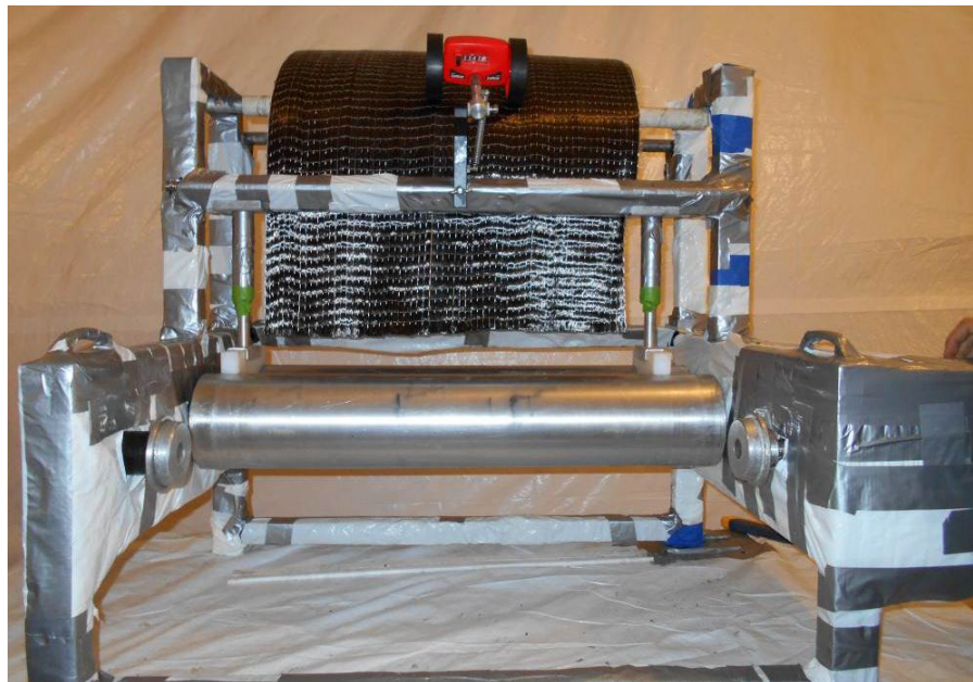
Figure 8 – Mechanical saturation equipment
