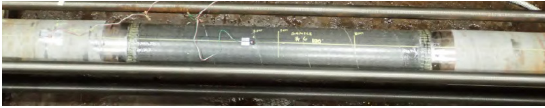
Figure 1: 8" diameter CFRP rehabilitation technology test specimen in axially restrained loading apparatus.
